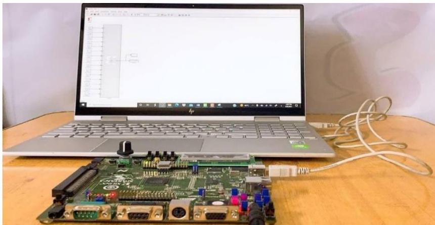
Figure 12. The connection setup of the laptop and the FPGA kit (Spartan-3A 700 A) through JTAG cable
