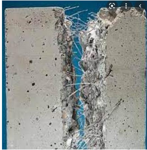
Figure 1. The role of fibres in reducing crack widening and redistributing it
