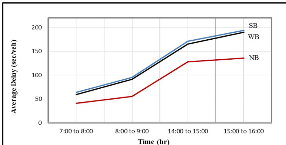
Figure 6. The average delay outputs of the current situation for the Andalus signaled intersection for vehicle traveling from EB to all approaches
