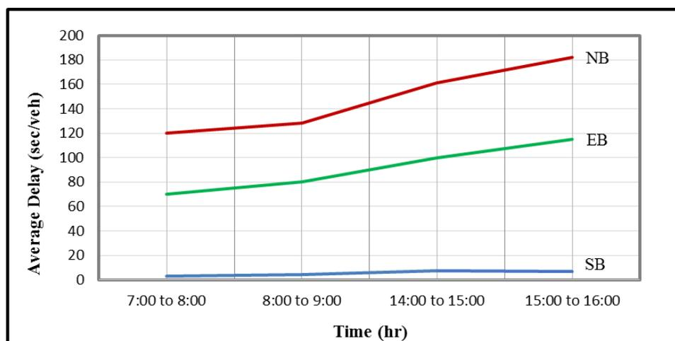
Figure 7. The average delay outputs of alteration No.1 for Andalus signalized intersection for vehicle traveling from WB to all Approaches
