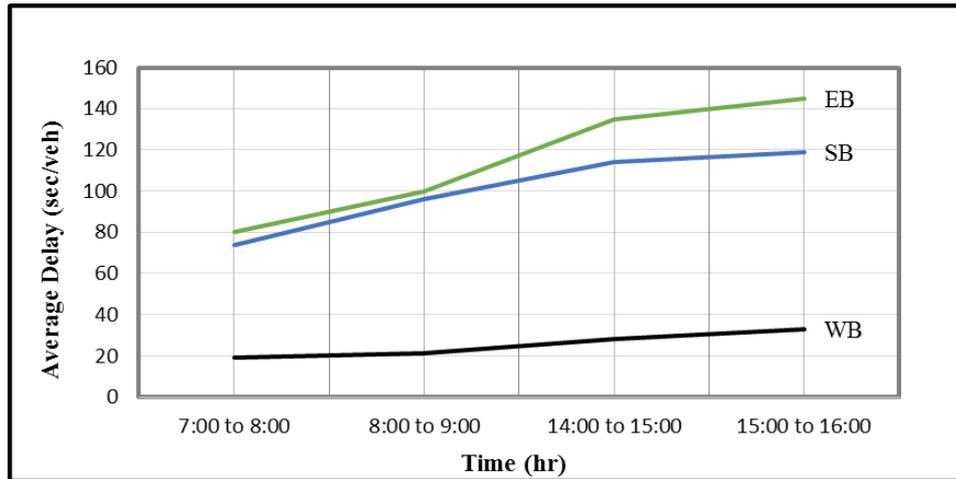
Figure 8. The average delay outputs of alteration No.1 for Andalus intersection for vehicle traveling from NB to all approaches
