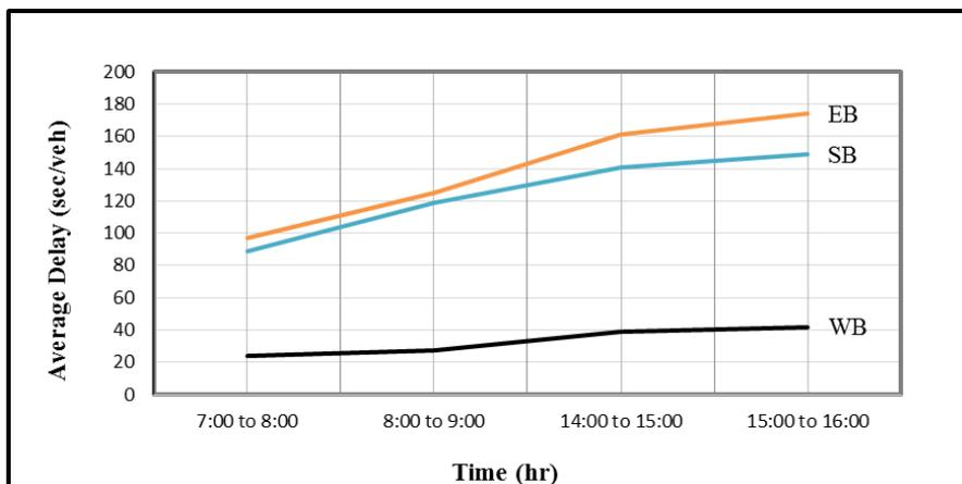
Figure 5. The average delay outputs of the current situation for the Andalus signaled intersection for vehicle traveling from NB to all approaches
