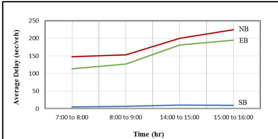
Figure 4. The average delay outputs of the Current Situation for the Andalus signaled intersection for vehicle traveling from WB to all approaches
