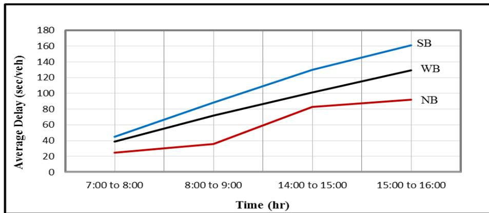
Figure 13. The average delay outputs of alteration No.2 for Andalus signalized intersection for vehicle traveling from EB to all approaches
