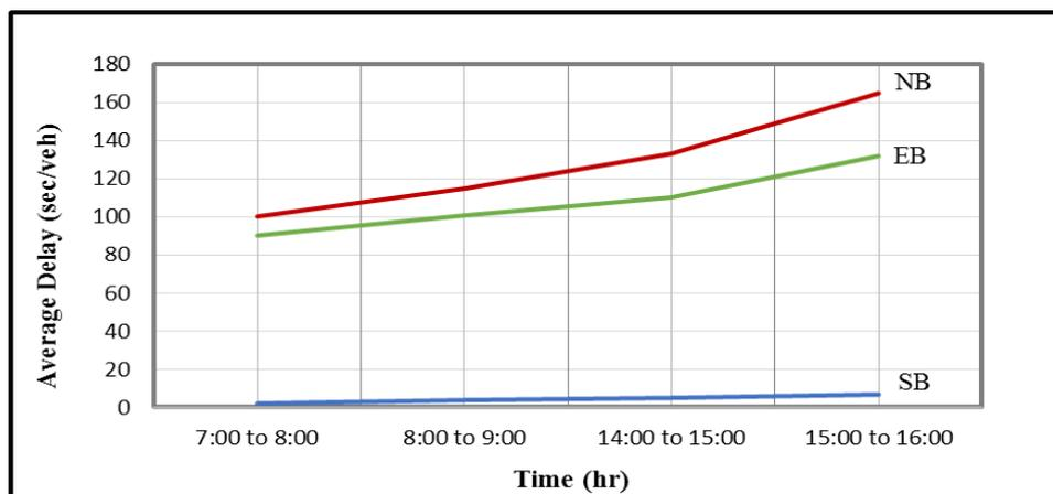
Figure 11. The average delay outputs of alteration No.2 for Andalus signalized intersection for vehicle traveling from WB to all Approaches
