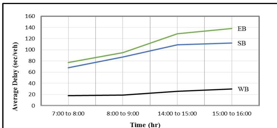
Figure 12. The average delay outputs of alteration No.2 for Andalus signalized intersection for vehicle traveling from NB to all approaches
