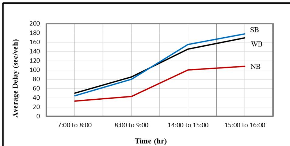
Figure 9. The average delay outputs of alteration No.1 for Andalus intersection for vehicle traveling from EB to all approaches
