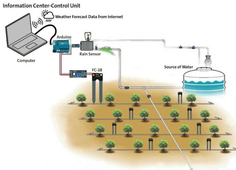
Figure 2. Mechanism of the irrigation system
