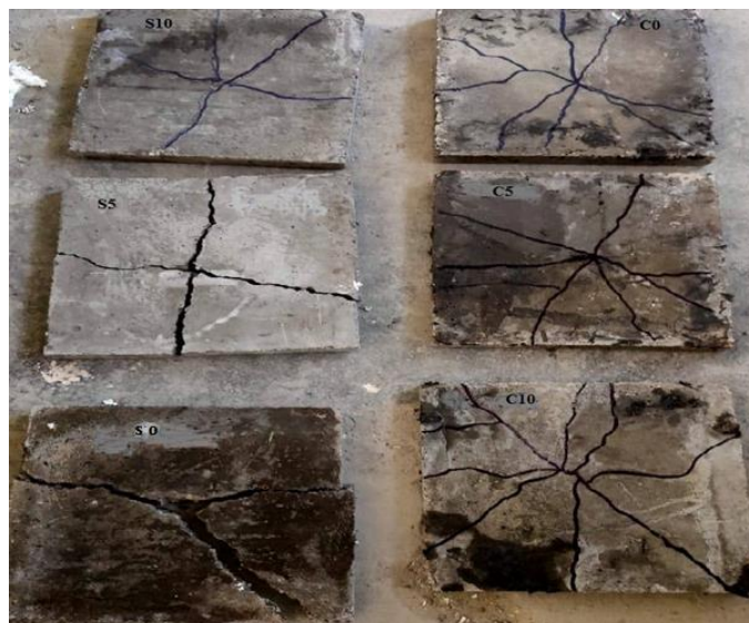
Figure 9. Cracking pattern of fixed supported ECC concrete for steel and carbon fiber
