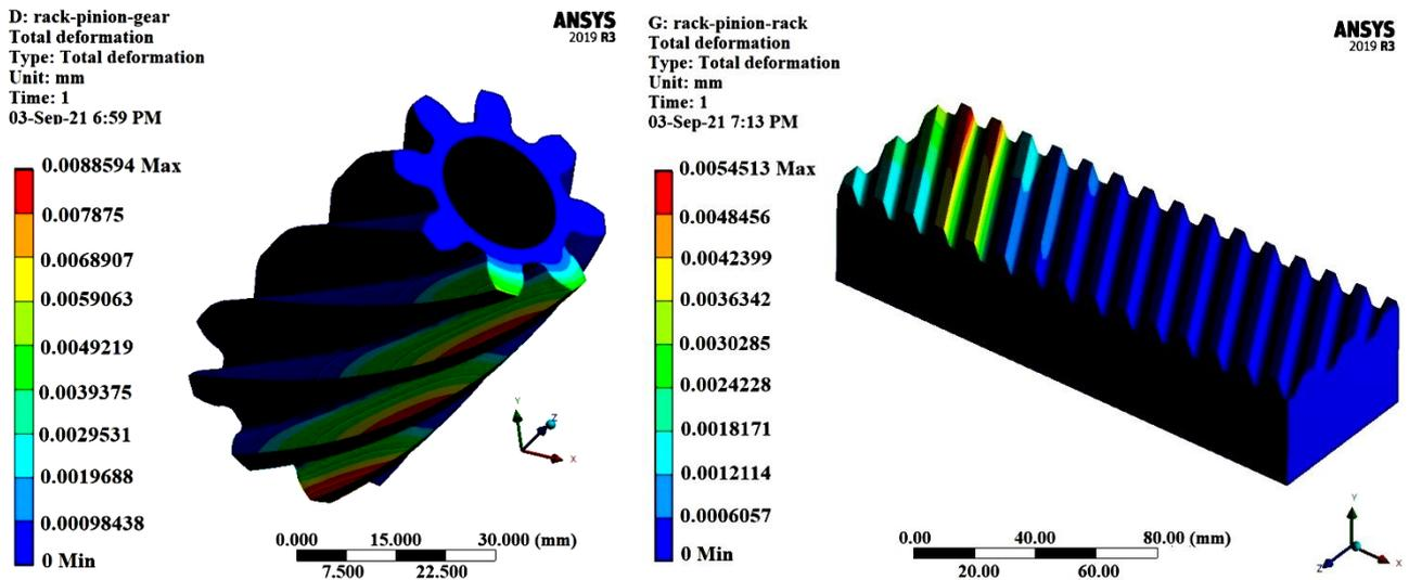
Figure 12.The total elastic deformation of rack-pinion (single helical gear)
