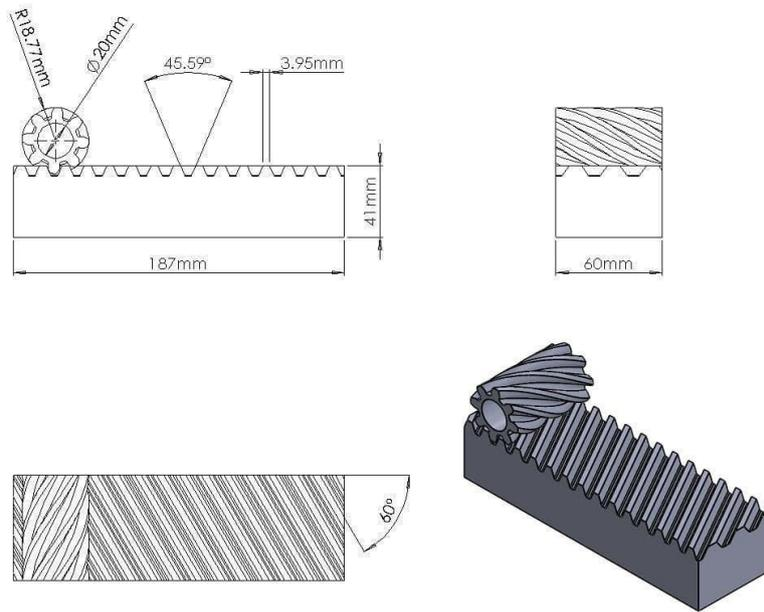
Figure 2. Shows the three projections and the final structure of the single helical gear (pinion) and rack
