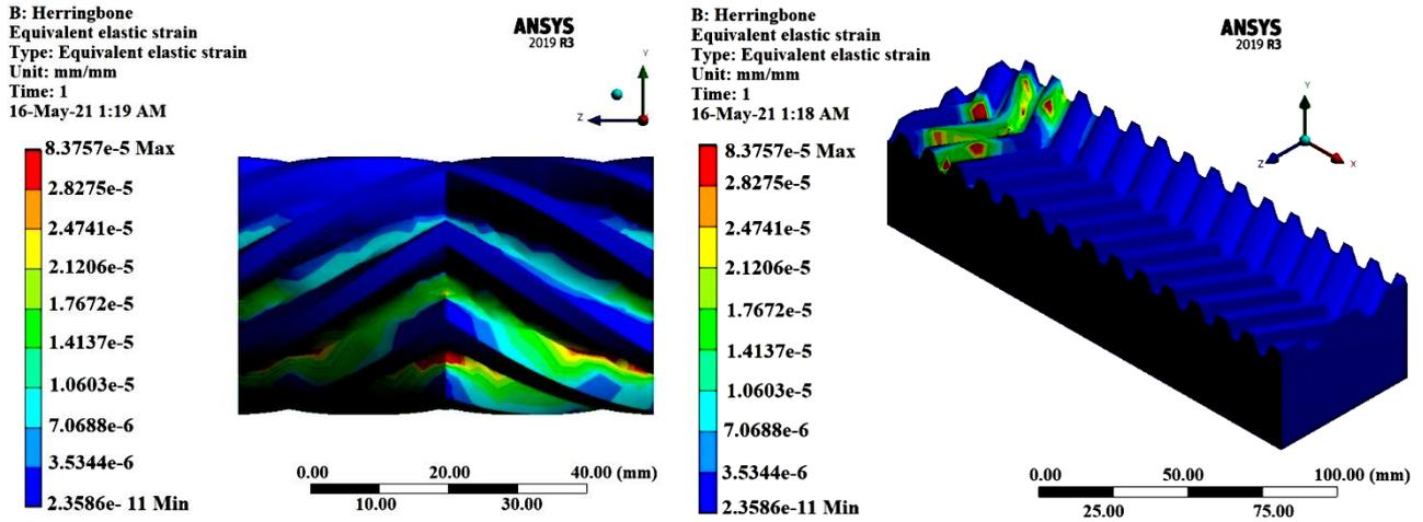
Figure 11.The strains of rack- pinion (herringbone gears)
