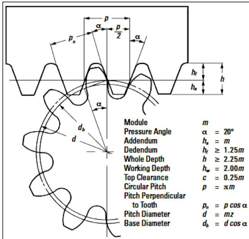
Figure 1. The tooth profile of rack and pinion [8]
