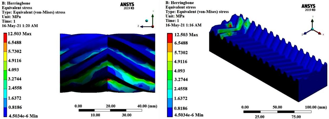
Figure 8. The distribution stresses of rack - pinion (herringbone gears)
