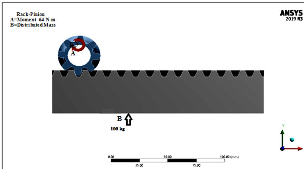
Figure 5. Shows the side view and the external loaded mass
