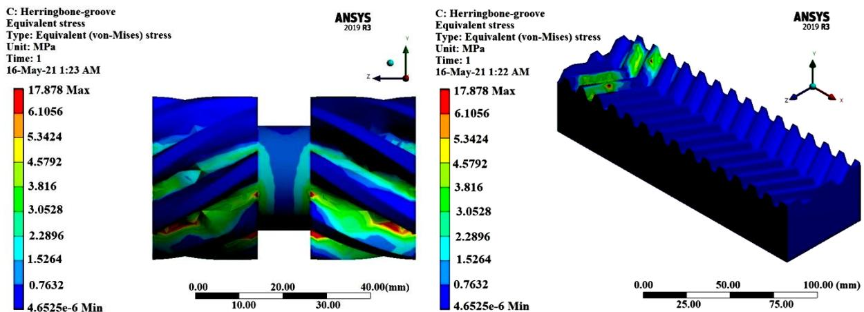
Figure 7. The distribution stresses of rack-pinion (double helical gear)
