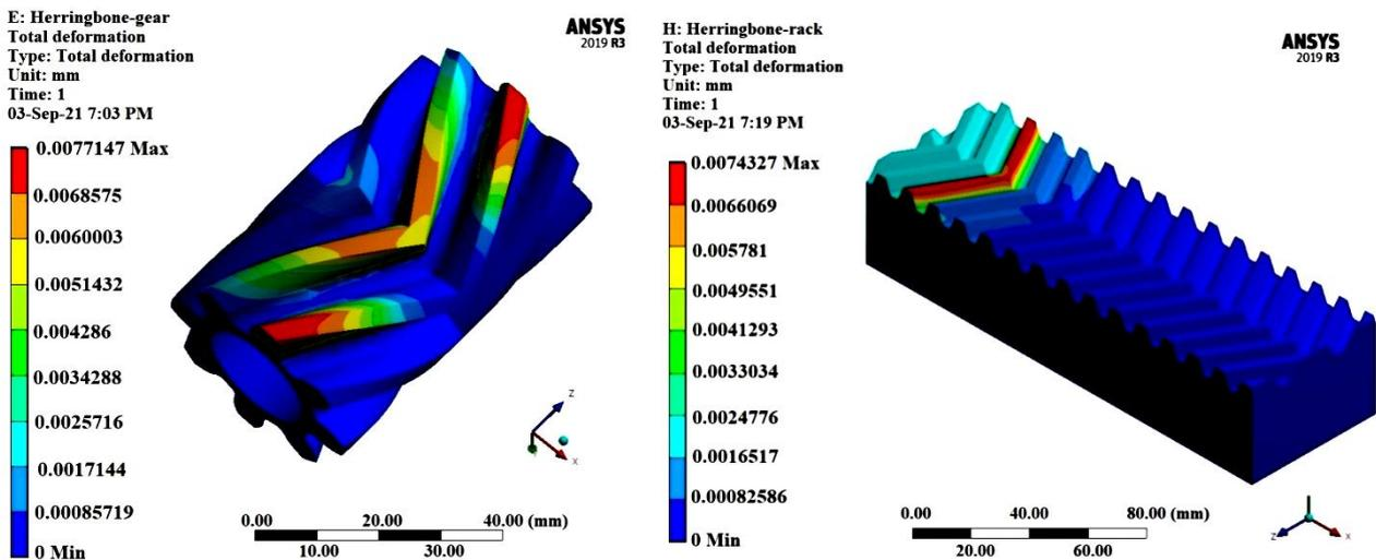
Figure 13.The total elastic deformation of rack-pinion (double helical gears)
