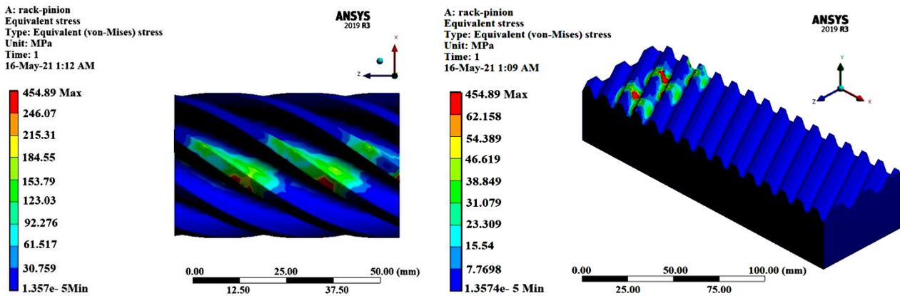
Figure 6. The distribution stresses of rack-pinion (single helical gear).
