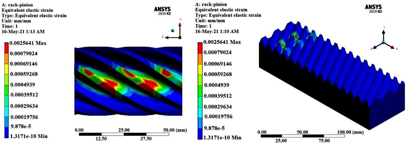
Figure 9. The strain of rack-pinion (single helical gear)
