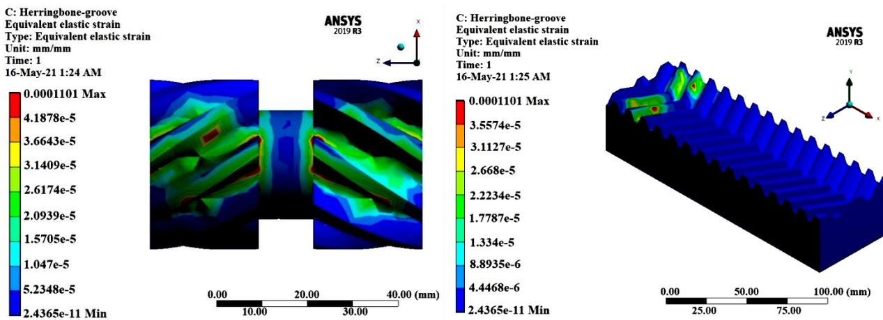
Figure 10. The strains of rack-pinion (double helical gears)
