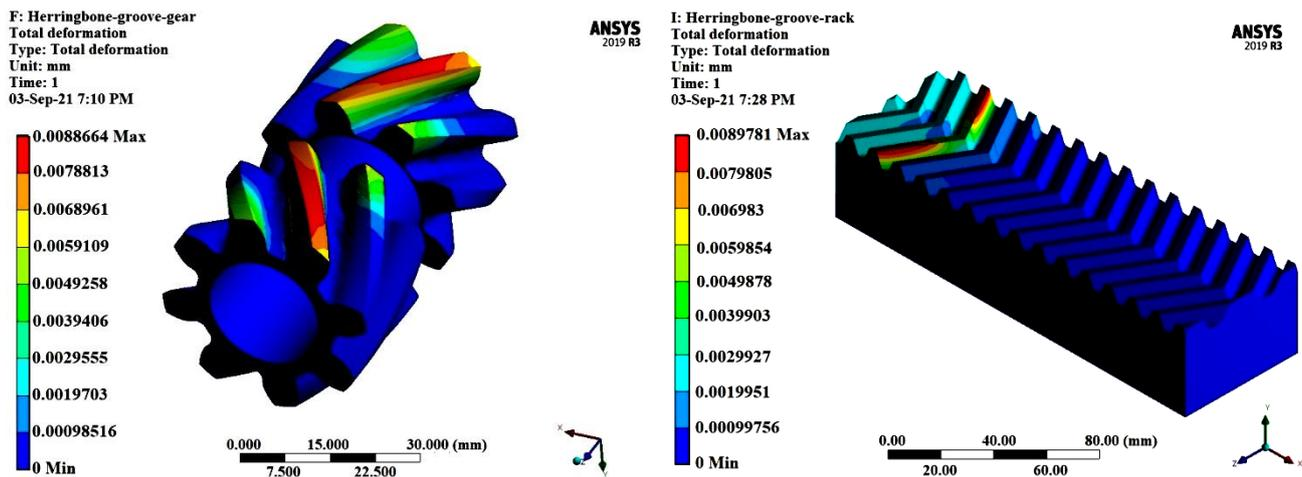
Figure 14 .The total elastic deformation of rack-pinion (herringbone gears)
