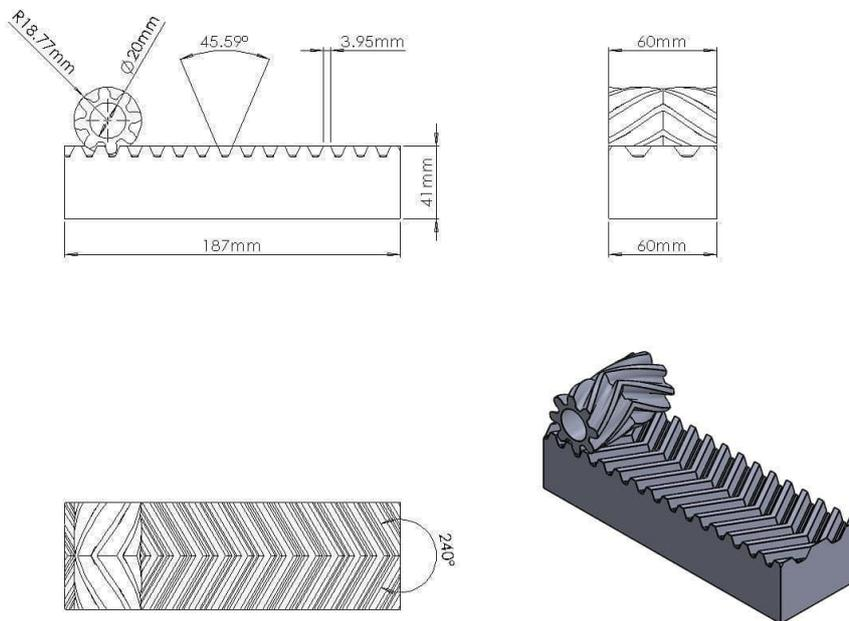
Figure 3. Shows the three projections and the final structure of the herringbone gear (pinion) and rack
