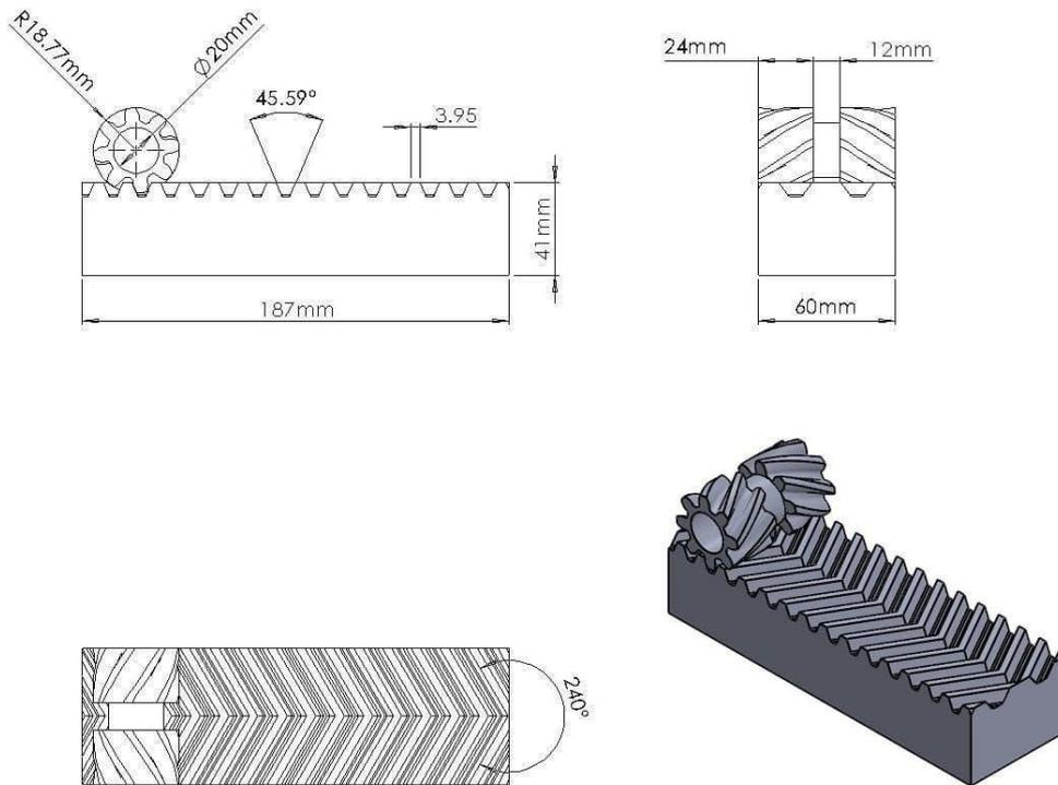
Figure 4. Shows the three projections and the final structure of double helical gear (pinion) and rack
