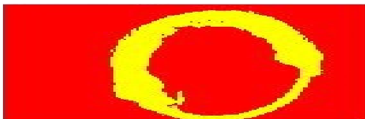
Figure 18. Segmenting the image (B2) by using Bernsen's Thresholding technique (B4)
