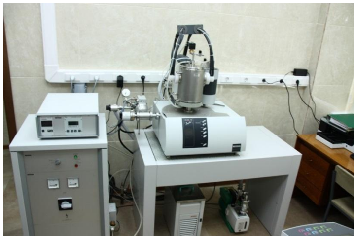
Figure 2. STA 449 F3 Jupiter device from NETZSCH (Germany).
