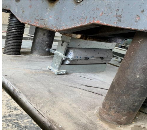
Figure 4. Splitting tensile test
