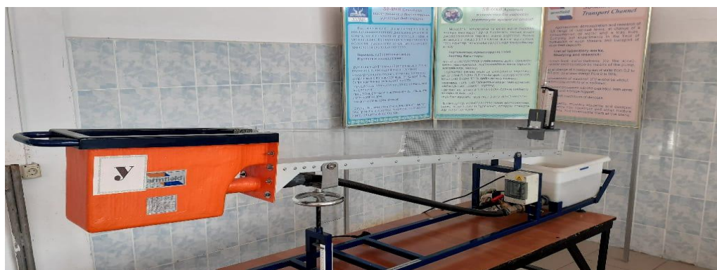
Figure 4. Installation (spillway channel) for conducting experiments in the field of hydraulics of open streams of the S8-MkII flume
