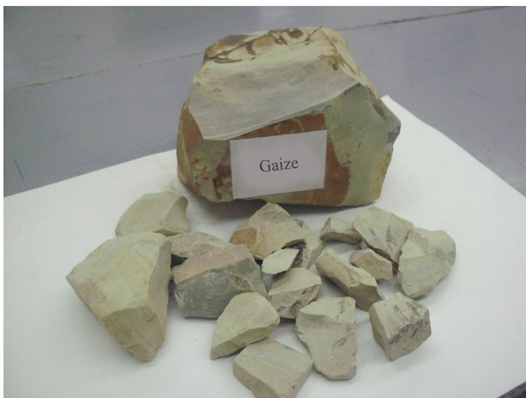
Figure 1. Gaize – siliceous rock of the West Kazakhstan deposit in its natural form
