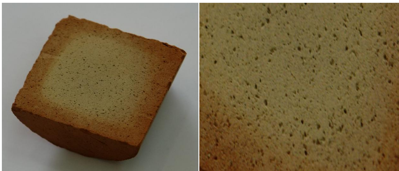
Figure 6. The porous macrostructure (in the cut) of heat-treated cylindrical samples at a temperature 1000°C
