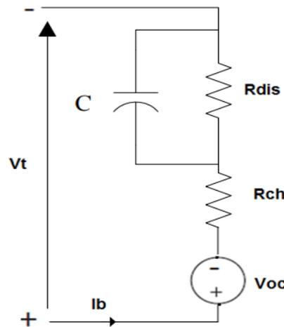
Figure 3. Simplifying model of battery
