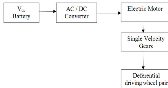
Figure 1. Battery electric Car power train scheme
