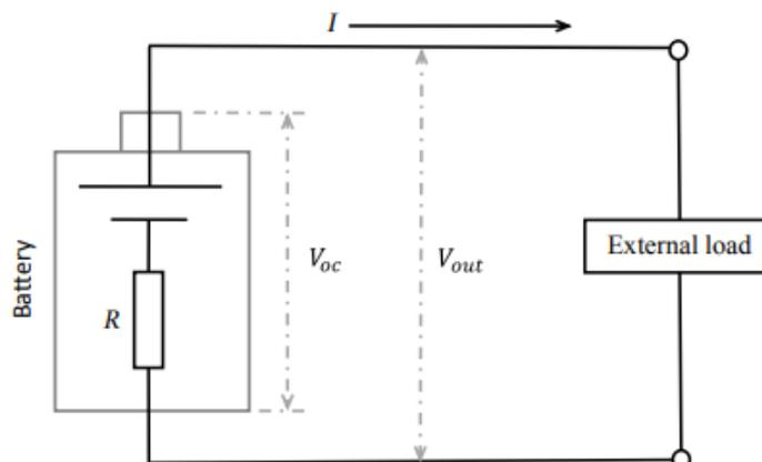
Figure 2. Modeling of equivalent circuit
