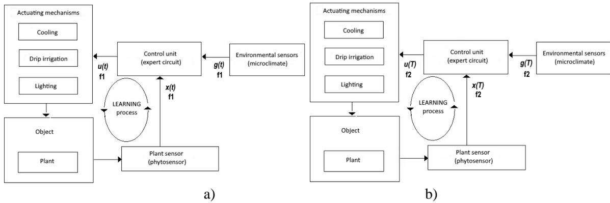
Figure 3. Control unit and data processing: a) in usage mode ( $f1$ ); b) in training mode ( $f2$ )
