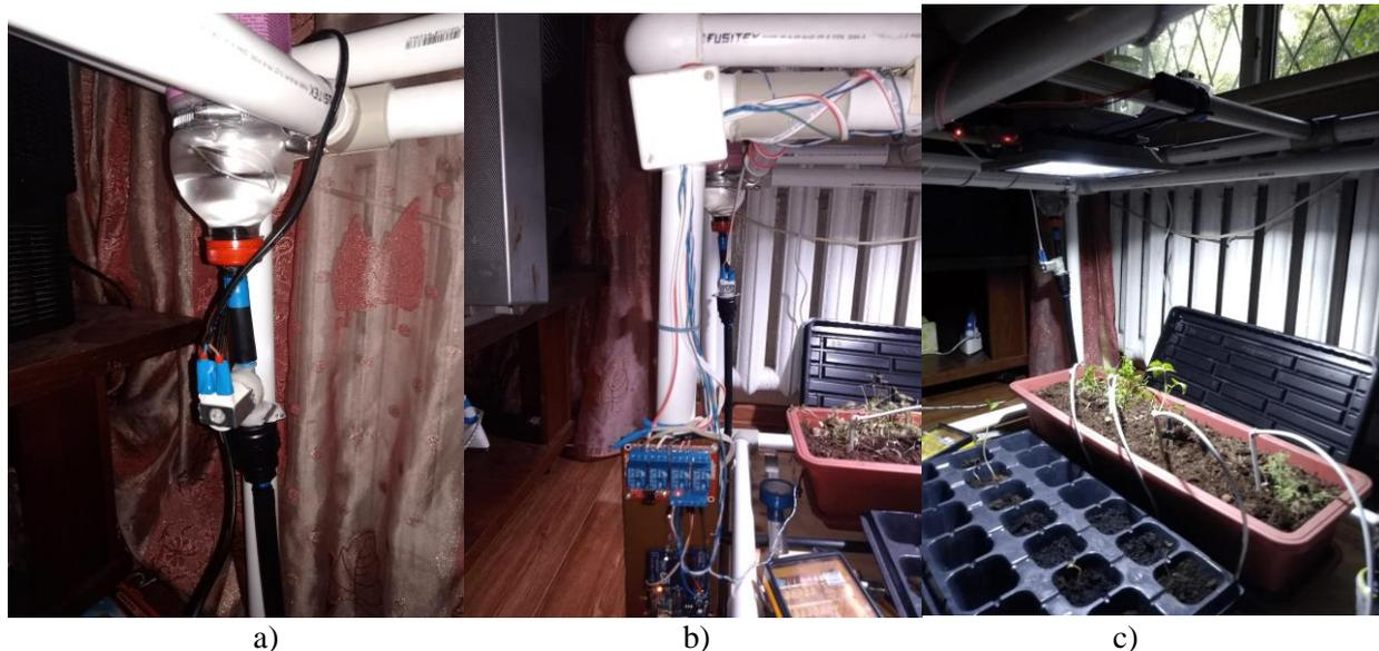
Figure 9. Home mini-greenhouse: a) irrigation valve; b) control unit; c) plants in the greenhouse
