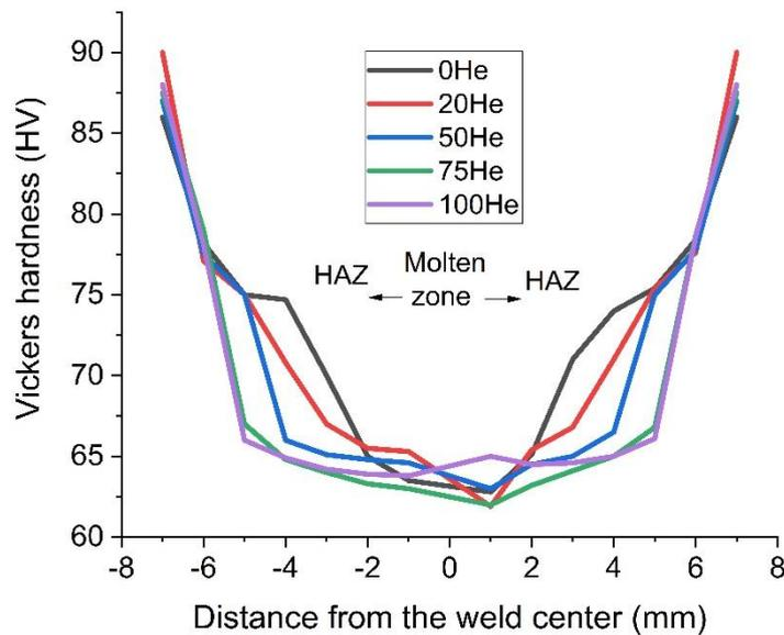
Figure 3. Microhardness distribution of welded joints
