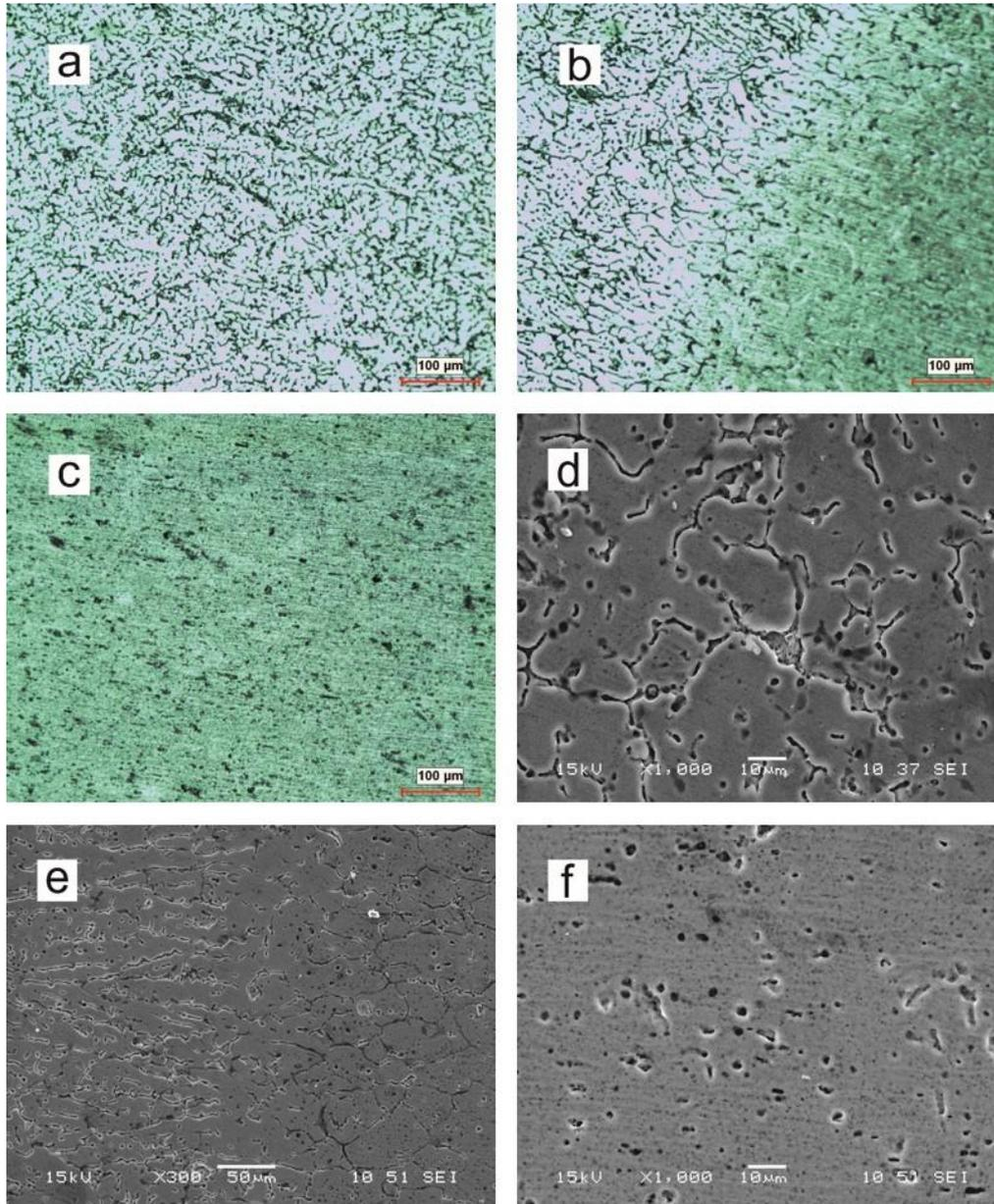
Figure 2. Images of optical (a) WM, b) HAZ, c) BM) and SEM (d) WM, e) HAZ, f) BM) microstructures of the section of 50He welded part
