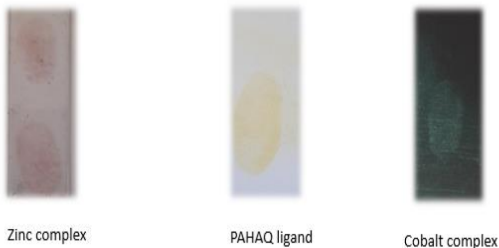
Figure 9. Detection of fingerprints by PAHQ ligand and its metal complexes of cobalt and zinc on smooth surface of glass
