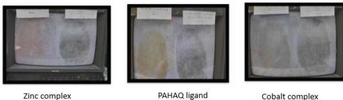
Figure 10. Comparison of fingerprints shown by PAHQ ligand and its metal complexes of zinc and cobalt with fingerprints shown by standard material (black ink)
