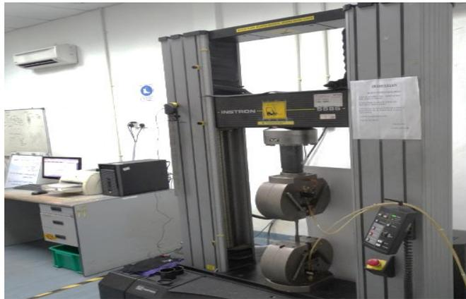
Figure 5. Tensile machine
