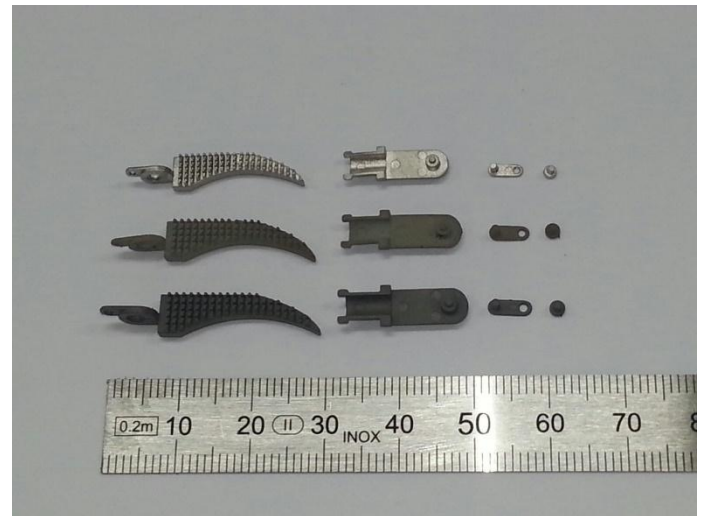
Figure 7. Green, brown, and sintered parts for the forcep of end-effector.
