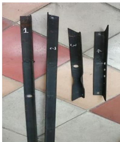
Figure 2. 1. Welding. 2. Shears.3. dubbed 4. Perforated.
