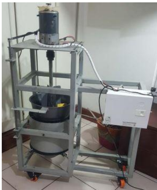
Figure 22. Functional prototype of the pulverized panela machine
