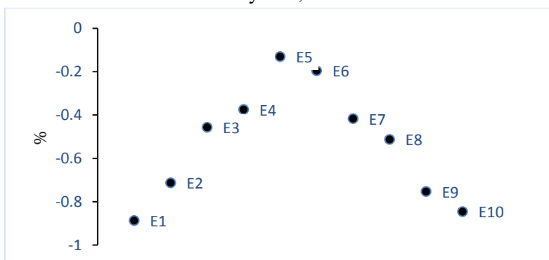
Figure 10. Graph of the average percentages of angular deviation of the mirrors comparing the positioning value of the control algorithm and the actual positioning of the system
