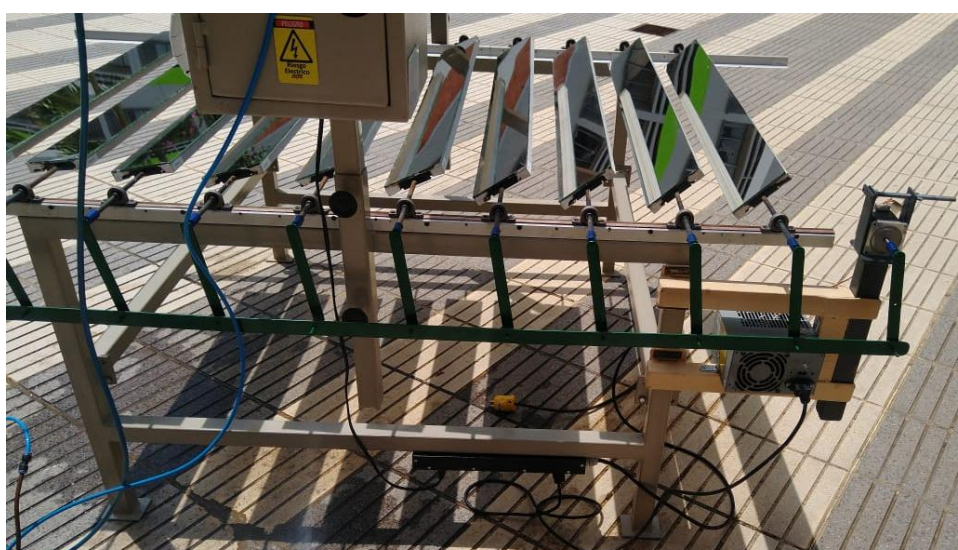
Figure 5. Full-scale mechanical system of the implemented solar tracking system
