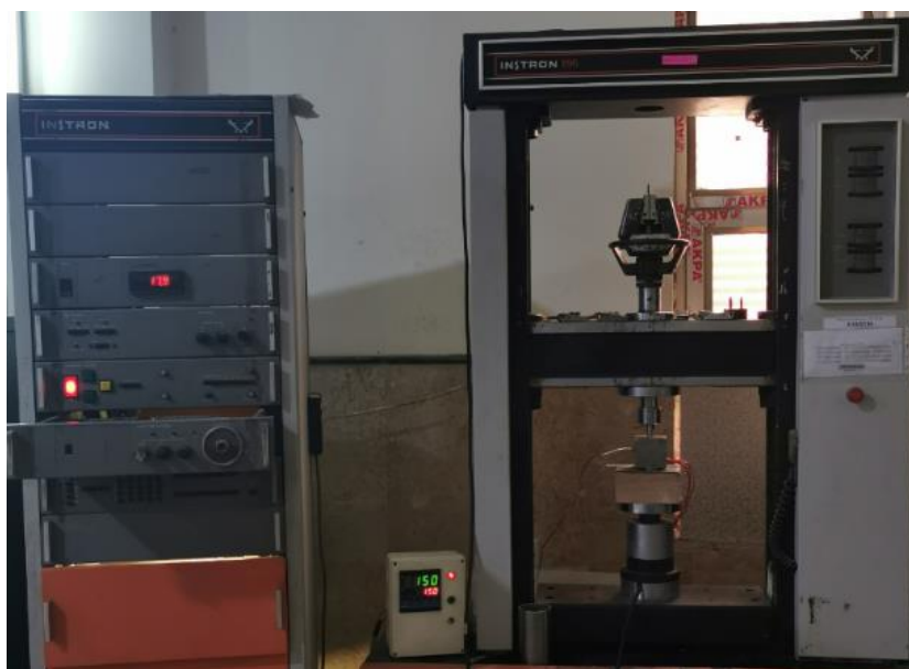
Figure 1. The hot Pressing System with Instron 1195 series
