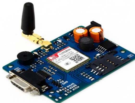
Figure 2. Shows the SIM800A Quad-Band GSM/GPRS Module with RS232 Interface
