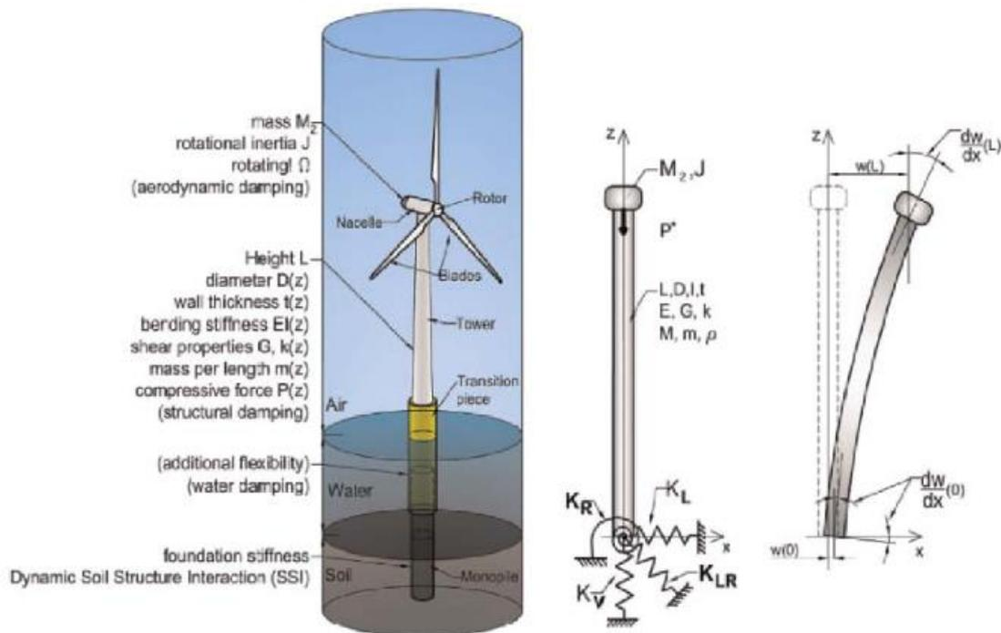
Figure 3. Simplified mechanical model of an OWT [29]
