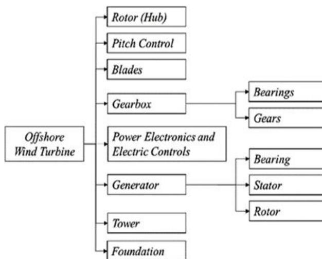
Figure 6. Subsystems and key components of an offshore wind turbine are broken down [35]
