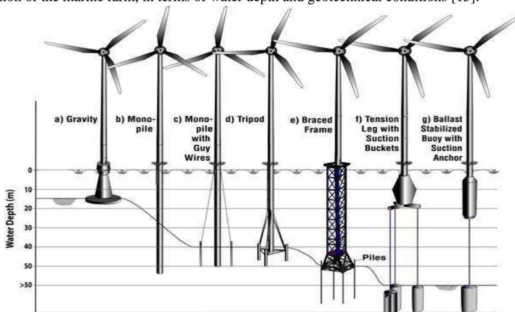
Figure 10. Support structure/foundation options for OWS, as well as their water depth requirements [70]
