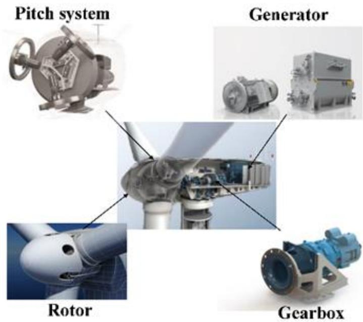
Figure 5. Components of the offshore wind turbine (OWT) system [34]
