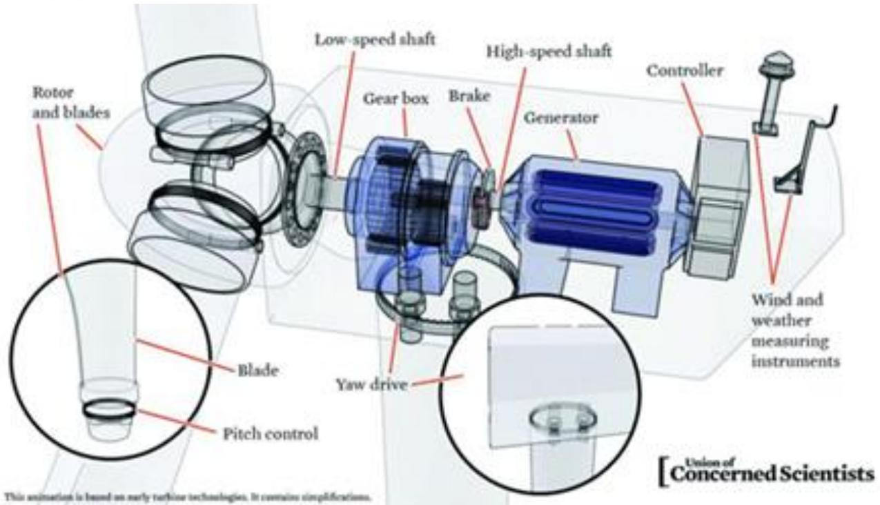
Figure 4. Components of an upwind-facing, horizontal-axis wind turbine with a gearbox motor, simplified [33]
