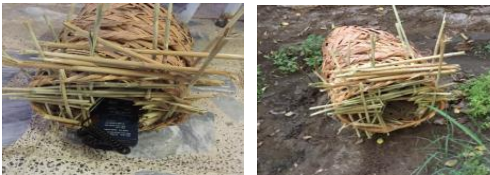
Figure 6. A model of (1/20) scale for a marsh cottage to measure temperature
