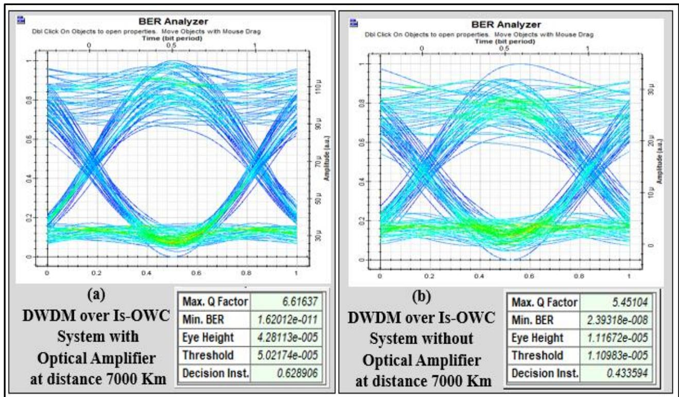
Figure 2. The eye diagrams, BER, and Q-Factor measurements for (a) DWDM over Is-OWC System with the optical amplifier at a distance 7000 Km (b) DWDM over Is-OWC system without optical amplifier at a distance 7000 Km
