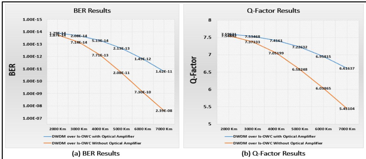
Figure 3. BER and Q-Factor results based on DWDM with and without Optical Amplifier over different Is-OWC distance
