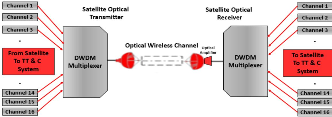
Figure 1. 16 Channels DWDM over Is-OWC system
