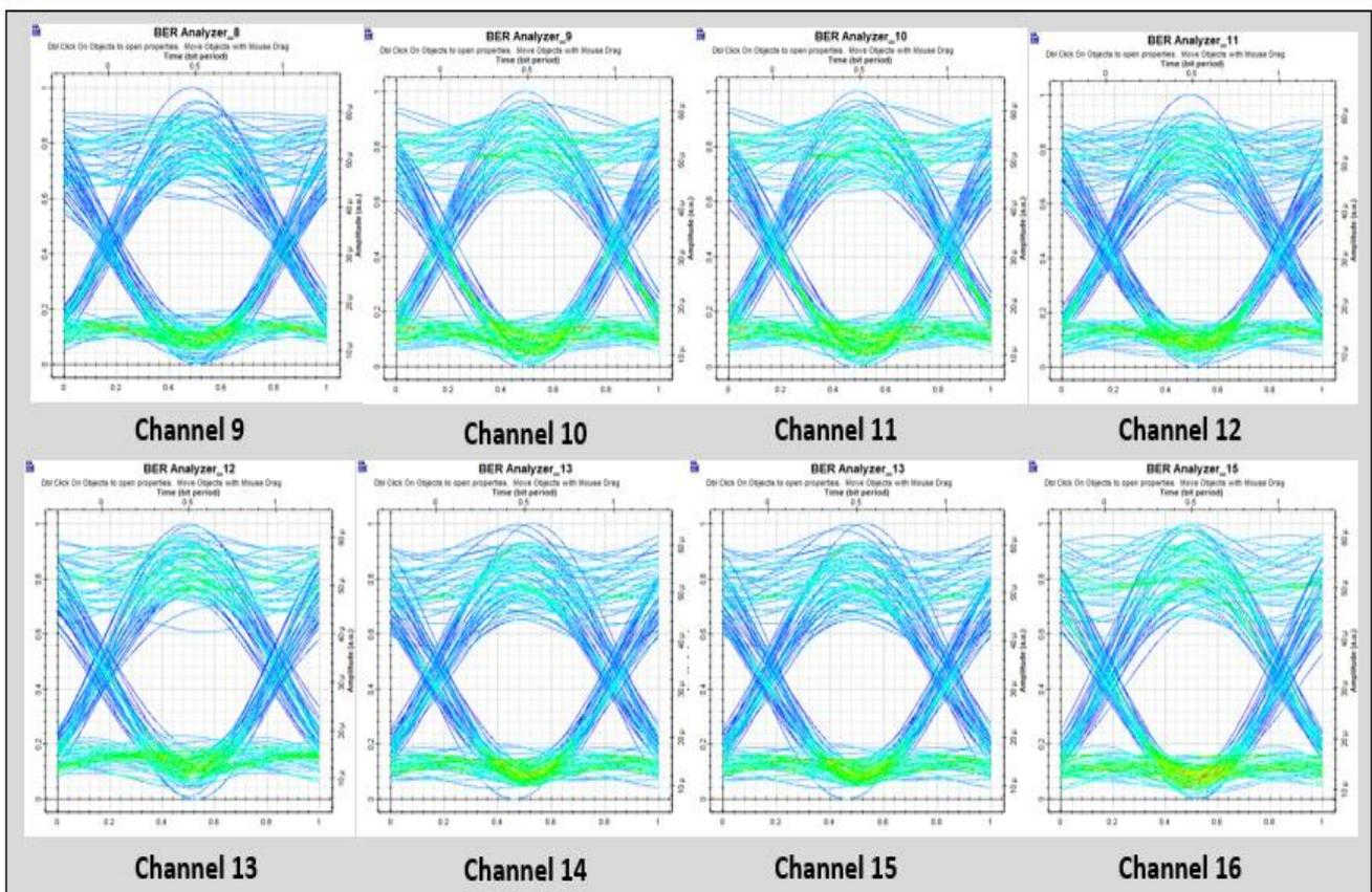
Figure 7. The eye diagrams measured for channel 9 to channel 16
