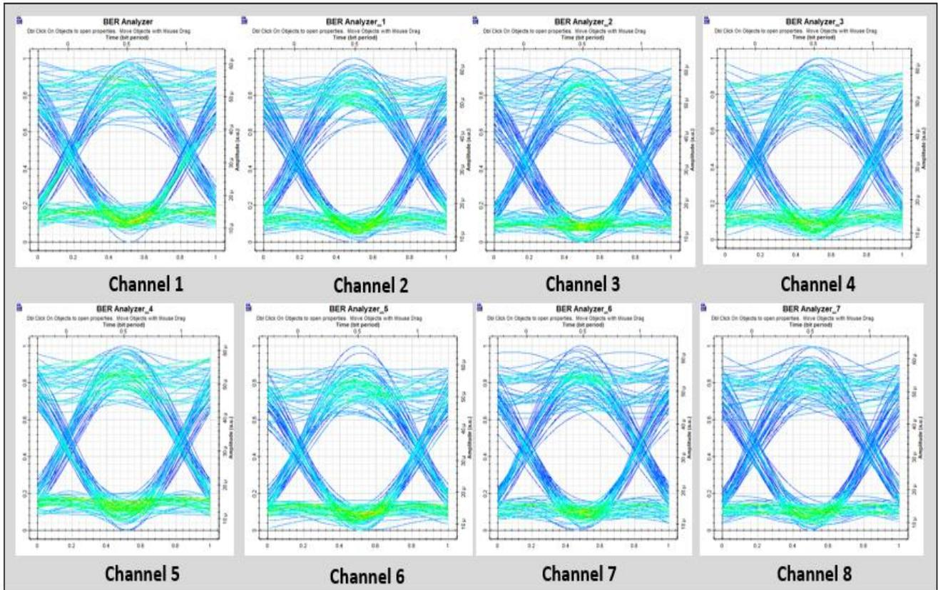
Figure 6. The eye diagrams measured for channel 1 to channel 8
