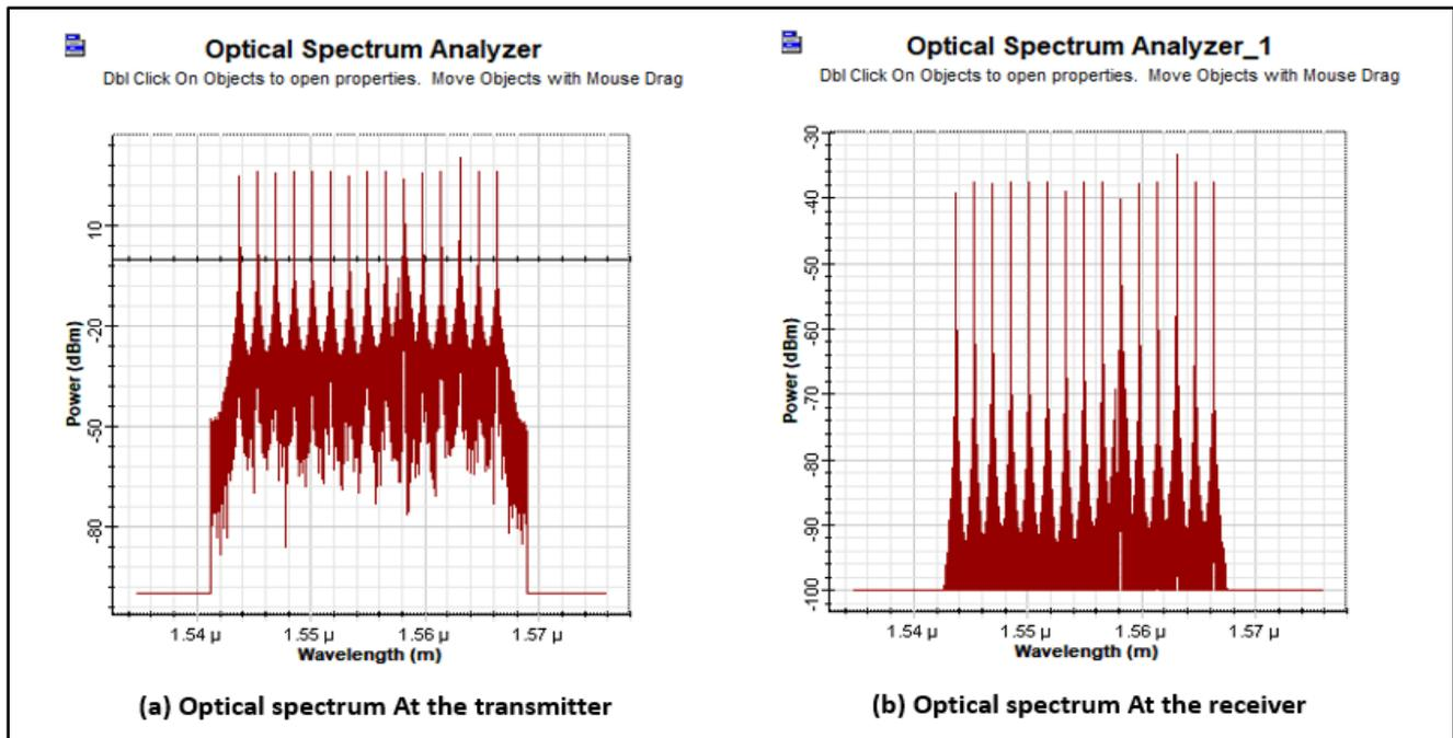
Figure 8. Optical spectrum under the influence of transmitting pointing error  $1.1 \mu\text{rad}$ .
