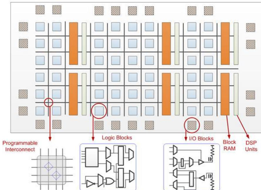
Figure 2. Internal component of FPGA
