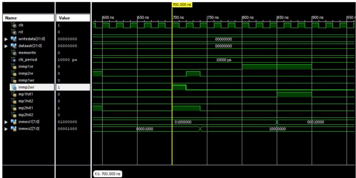
Figure 10. Test bench of MESI protocol-MP1 Hit Write (Direct Write).
