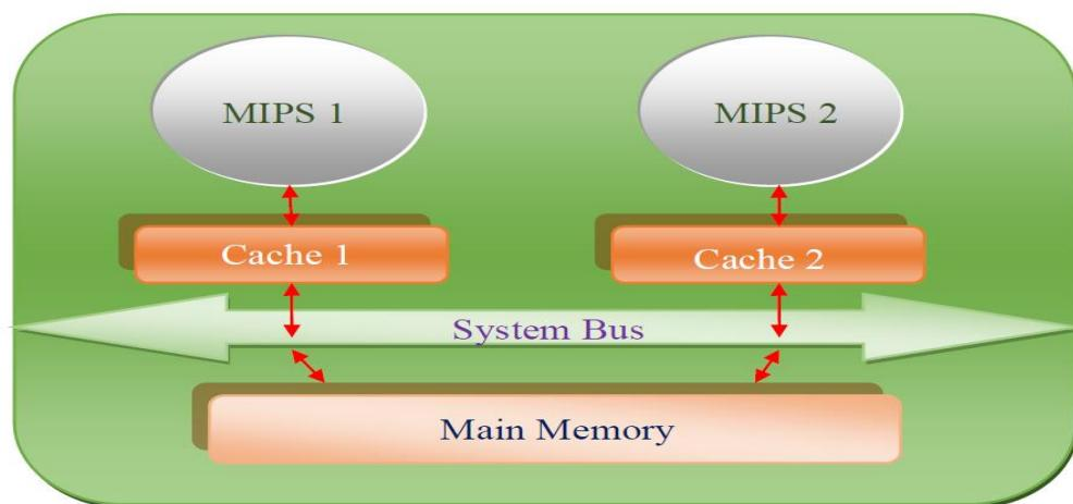
Figure 3. Architecture of dual microprocessor
