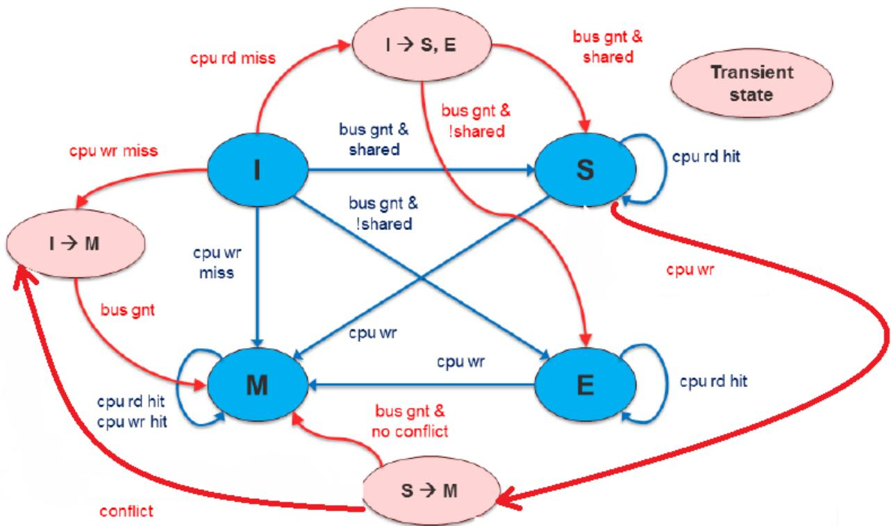
Figure 6. Simple MESI state diagram with state transfer
