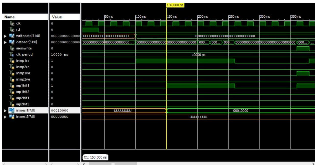
Figure 9. Test bench of MESI protocol-MP1 Hit Read (Direct Read)
