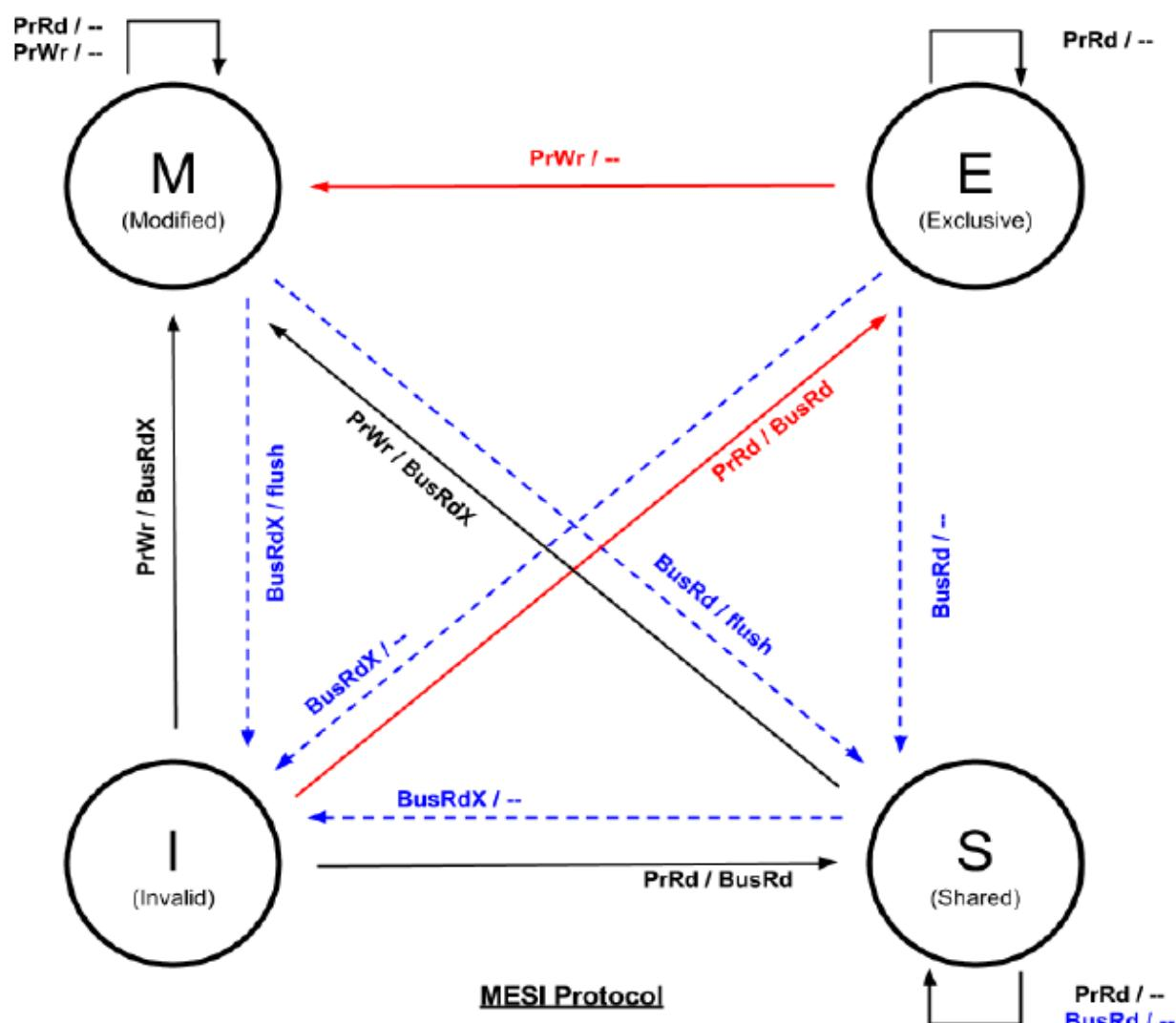
Figure 5. State transition diagram for the MESI protocol
