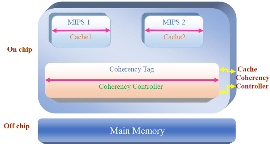
Figure 7. Block diagram for the cache coherency controller
