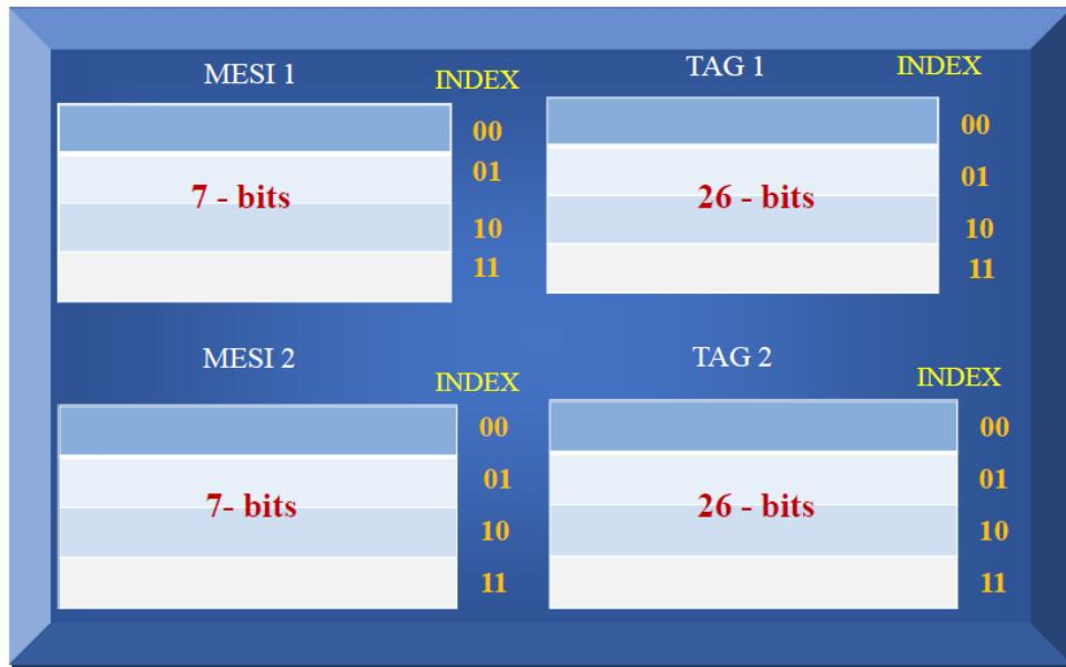
Figure 8. Coherency tag with 7-bits for MESI states
