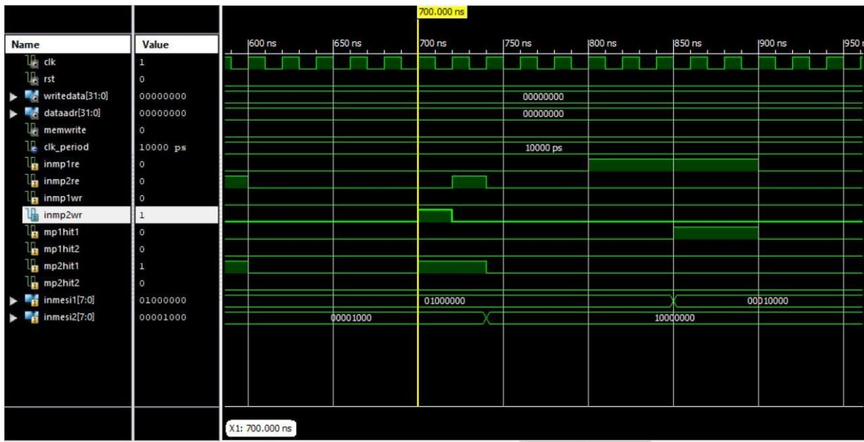
Figure 10. Test bench of MESI protocol-MP1 Hit Write (Direct Write).
