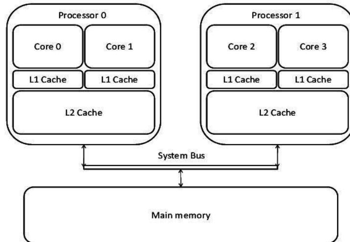
Figure 1. Dual multicore processor.
