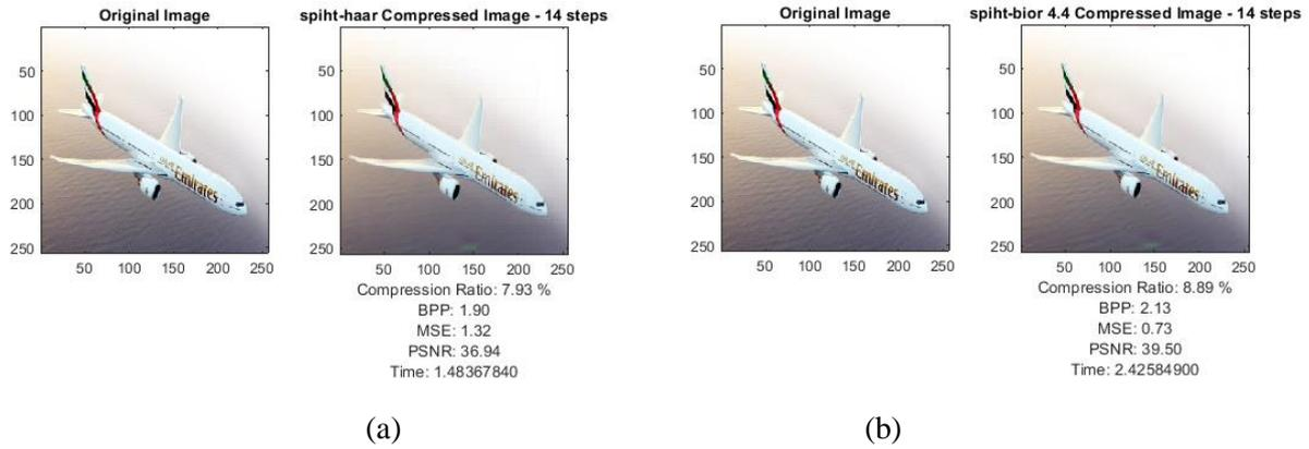
Figure 4. The result of (a) 1<sup>st</sup> compression by using spiht compression algorithm based on Bior 4.4 wavelet method, and (b) 2<sup>nd</sup> compression by using spiht compression algorithm based on Haar wavelet method. With number of coding = 14 loop
