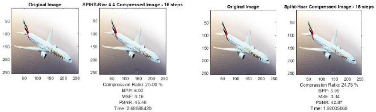
Figure 14. The result of (a) 1<sup>st</sup> compression by using spiht compression algorithm based on Bior 4.4 wavelet method, and (b) 2<sup>nd</sup> compression by using spiht compression algorithm based on Haar wavelet method. With number of coding = 16 loop
