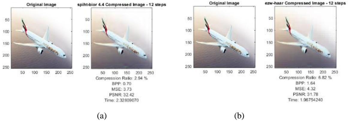
Figure 7. The result of (a) 1<sup>st</sup> compression by using spiht compression algorithm based on Bior 4.4 wavelet method, and (b) 2<sup>nd</sup> compression by using ezw compression algorithm based on Haar wavelet method. With number of coding = 12 loop
