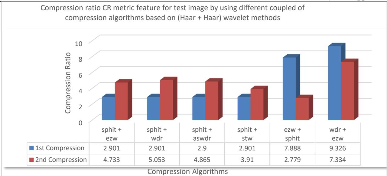
Figure 19. The bar chart of the compression ratio for test image by using different coupled compression algorithms based on (Haar + Haar) wavelet methods
