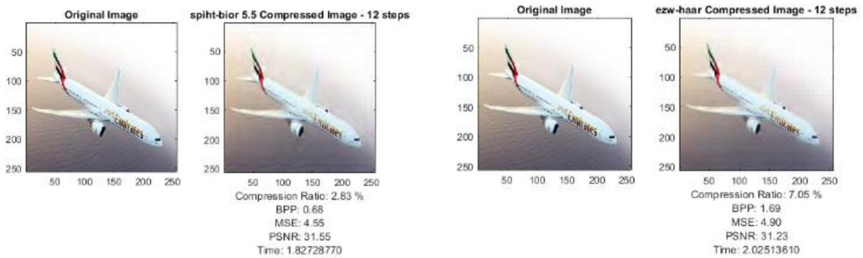
Figure 8. The result of (a) 1<sup>st</sup> compression by using spiht compression algorithm based on Bior 5.5 wavelet method, and (b) 2<sup>nd</sup> compression by using ezw compression algorithm based on Haar wavelet method. With number of coding = 12 loop
