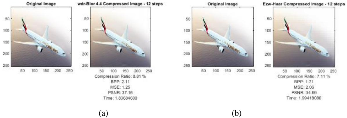
Figure 10. The result of (a) 1<sup>st</sup> compression by using wdr compression algorithm based on Bior 4.4 wavelet method, and (b) 2<sup>nd</sup> compression by using ezw compression algorithm based on Haar wavelet method. With 12 loop
