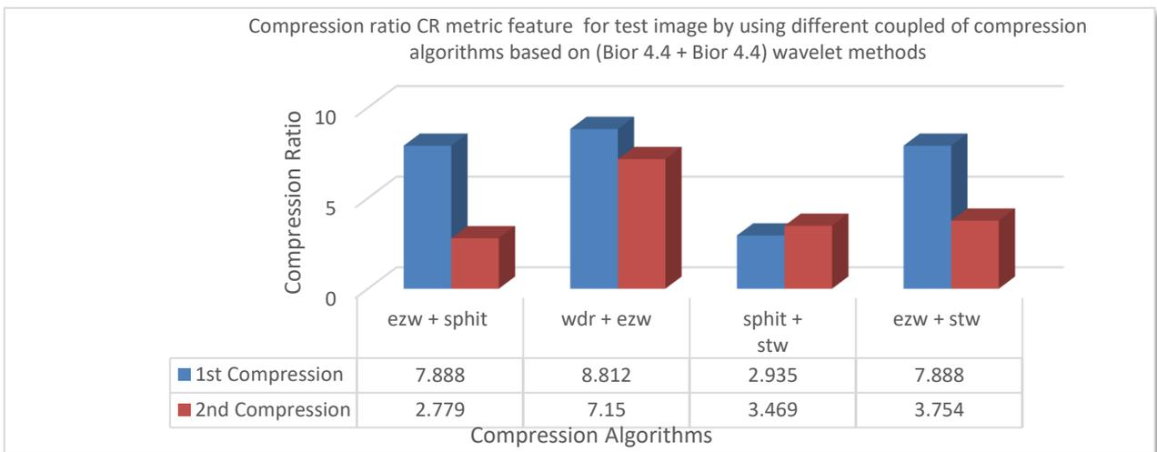
Figure 20. The bar chart of the compression ratio for test image by using different coupled compression algorithms based on (Bior 4.4 + Bior 4.4) wavelet methods
