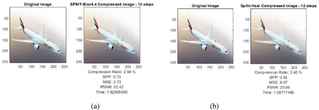
Figure. 12. The result of (a) 1<sup>st</sup> compression by using spiht compression algorithm based on Bior 4.4 wavelet method, and (b) 2<sup>nd</sup> compression by using spiht compression algorithm based on Haar wavelet method. With number of coding = 12 loop
