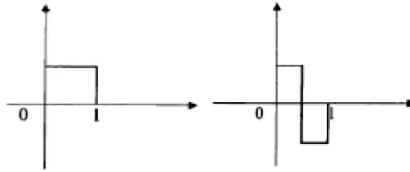
Figure 1. The HAAR scaling and wavelet functions [14]
