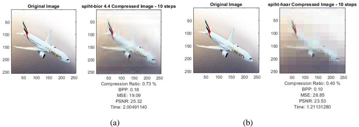
Figure 6. The result of (a) 1<sup>st</sup> compression by using spiht compression algorithm based on Bior 4.4 wavelet method, and (b) 2<sup>nd</sup> compression by using spiht compression algorithm based on Haar wavelet method. With number of coding = 10 loop
