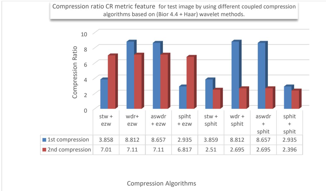
Figure 17. The bar chart of the compression ratio for test image by using different coupled compression algorithms based on (Bior 4.4 + Haar) wavelet methods
