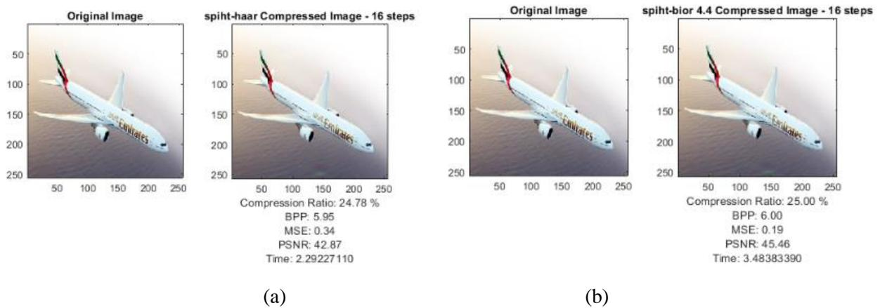
Figure 5. The result of (a) 1<sup>st</sup> compression by using spiht compression algorithm based on Bior 4.4 wavelet method, and (b) 2<sup>nd</sup> compression by using spiht compression algorithm based on Haar wavelet method. With number of coding = 16 loop
