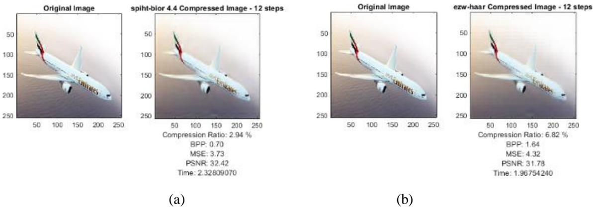
Figure 11. The result of (a) 1<sup>st</sup> compression by using spiht compression algorithm based on Bior 4.4 wavelet method, and (b) 2<sup>nd</sup> compression by using ezw compression algorithm based on Haar wavelet method. With 12 loop
