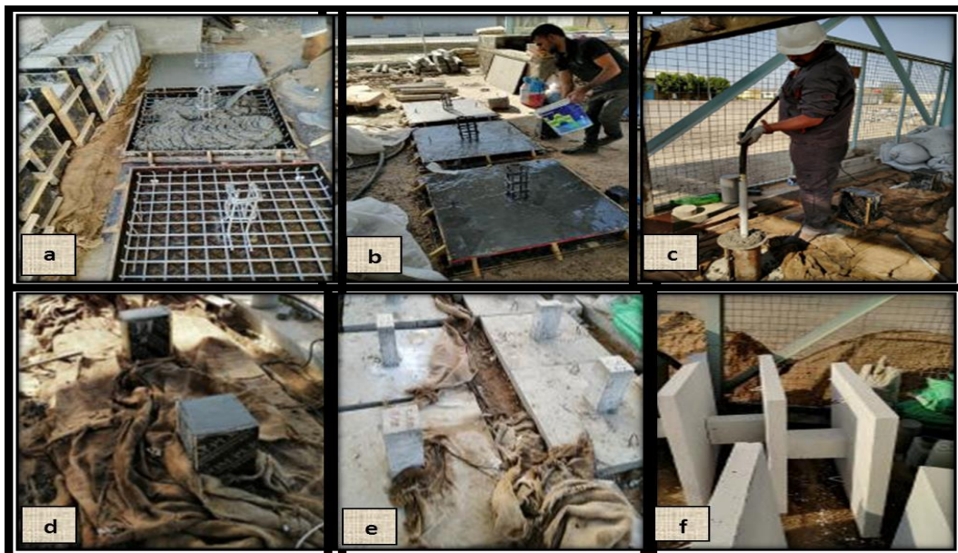
Figure 5. Samples, casting and curing
