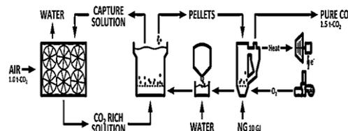
Figure 1. Carbon engineering's air captures process
