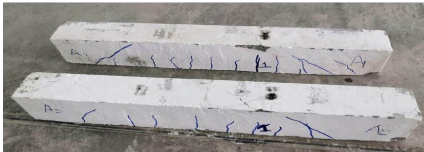
Figure 9. Experimental work Crack pattern [2]
