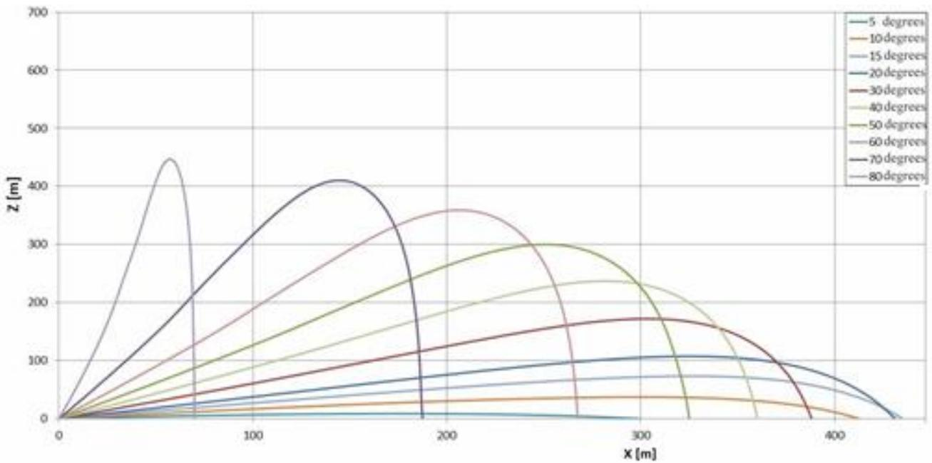
Figure 7. Trajectories of the fragment (7.89g) in the plane x-z
