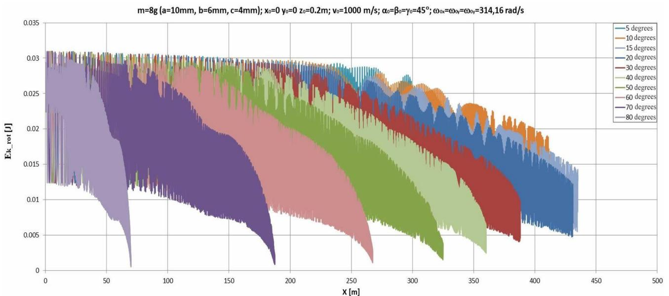
Figure 14. Decrease of rotational kinetic energy for 7.89g fragment for different elevation angles
