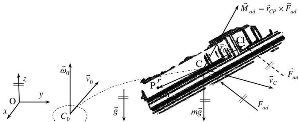
Figure 2. Free body diagram of the fragment and equivalent force and moment acting at the center of gravity
