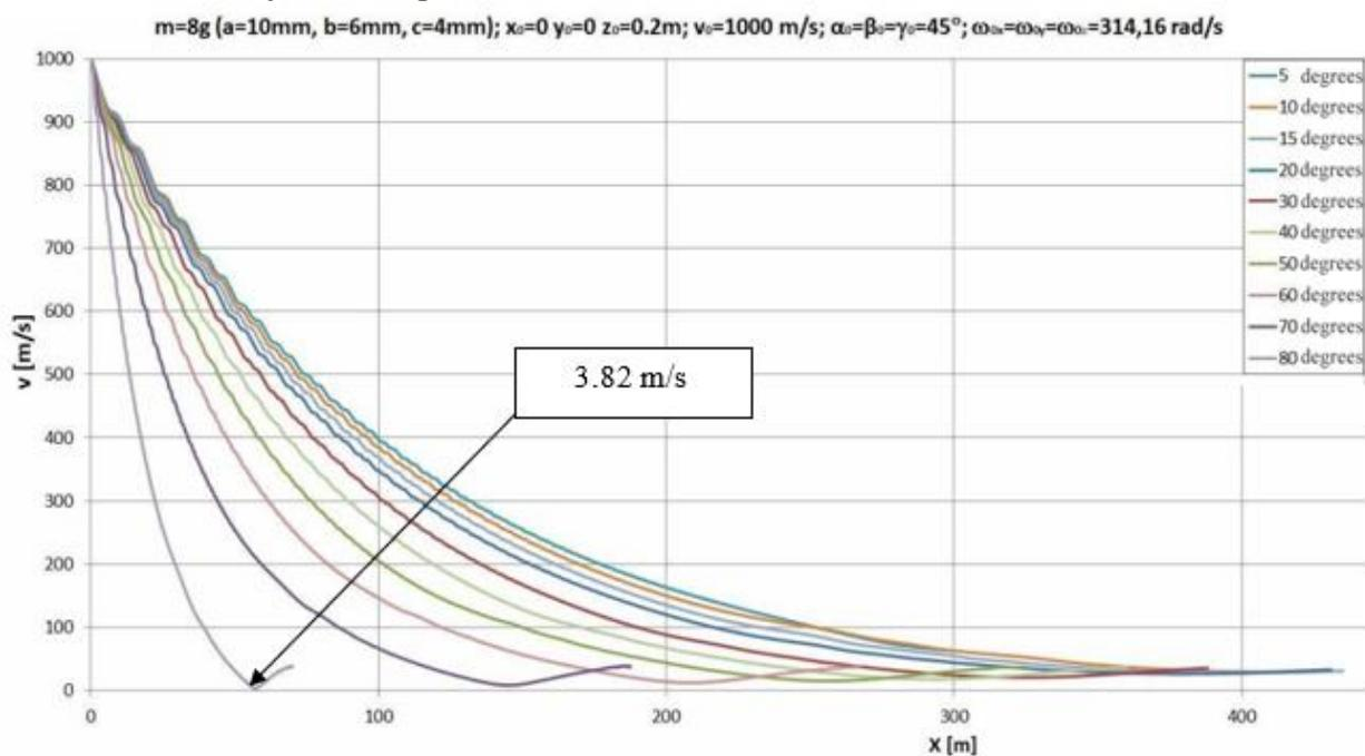
Figure 11. Change of the translational velocity intensity for the different elevation angles
