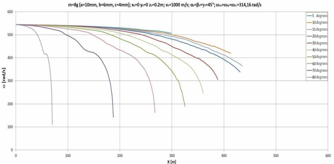
Figure 10. Changes in the intensity of angular velocity for the different elevation angles
