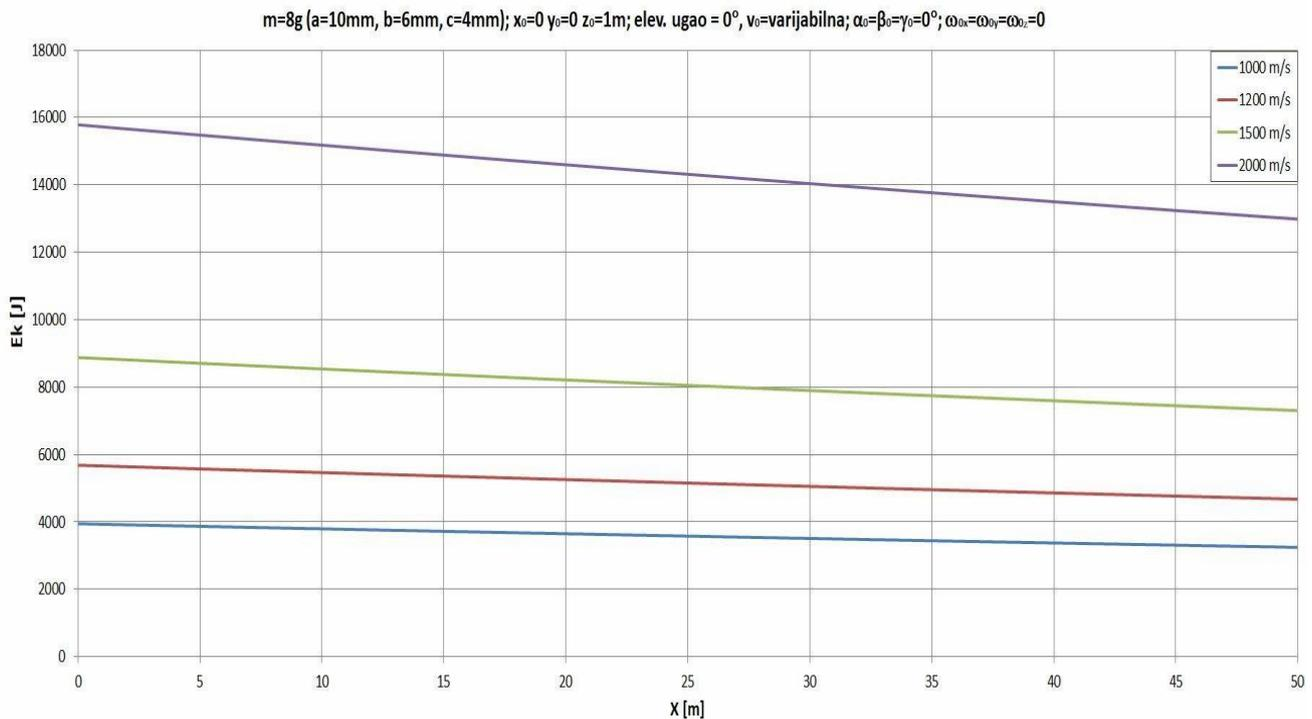
Figure 16. Change of the kinetic energy for the given fragment (mass of 7.89g) for different initial translational velocities, up to a distance of 50m.
