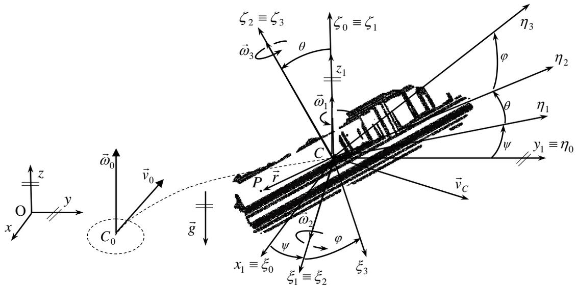
Figure 3. Visualization of coordinate systems and kinematic parameters during the movement of fragment through the resistive medium
