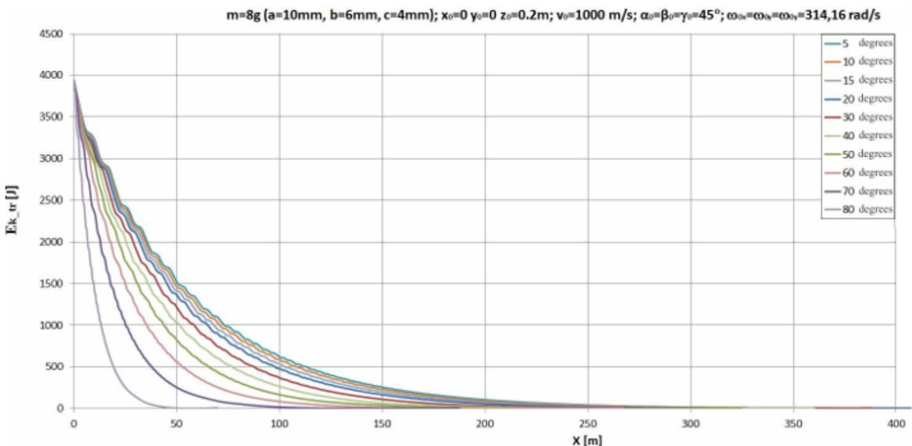
Figure 12. Decrease of translational kinetic energy for a fragment with a mass of 7.89 g for different elevation angles
