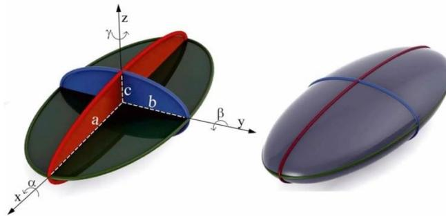
Figure 5. Initial zero position of the ellipsoidal body in the Matlab program for the calculation of irregularly shaped body trajectory
