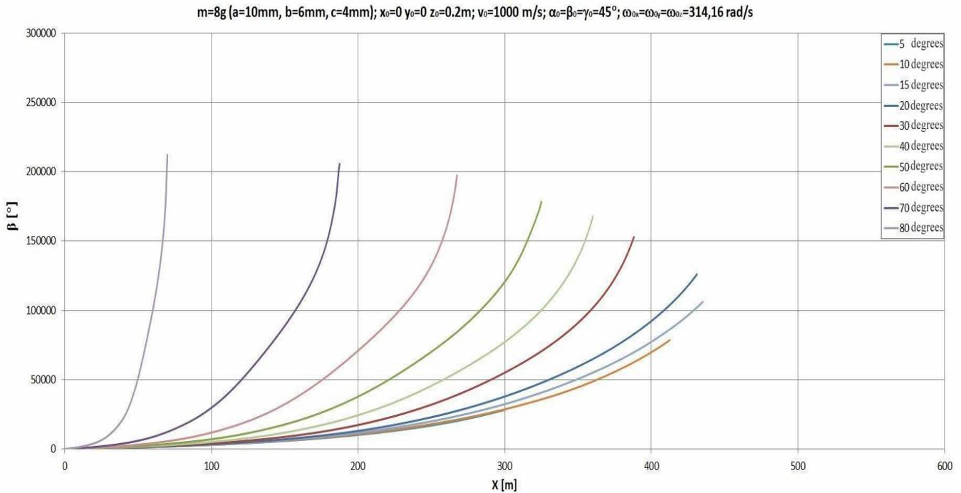
Figure 9. Change of the pitch angle  $\beta$  (rotation around axis y) as a function of distance
