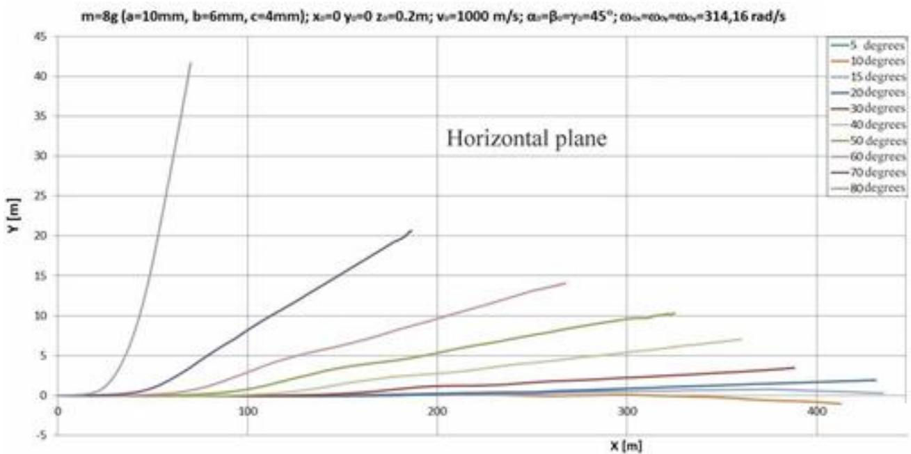
Figure 8. Lateral (side) movement (in the x-y plane) of the fragment with mass 7.89g for different elevation angles
