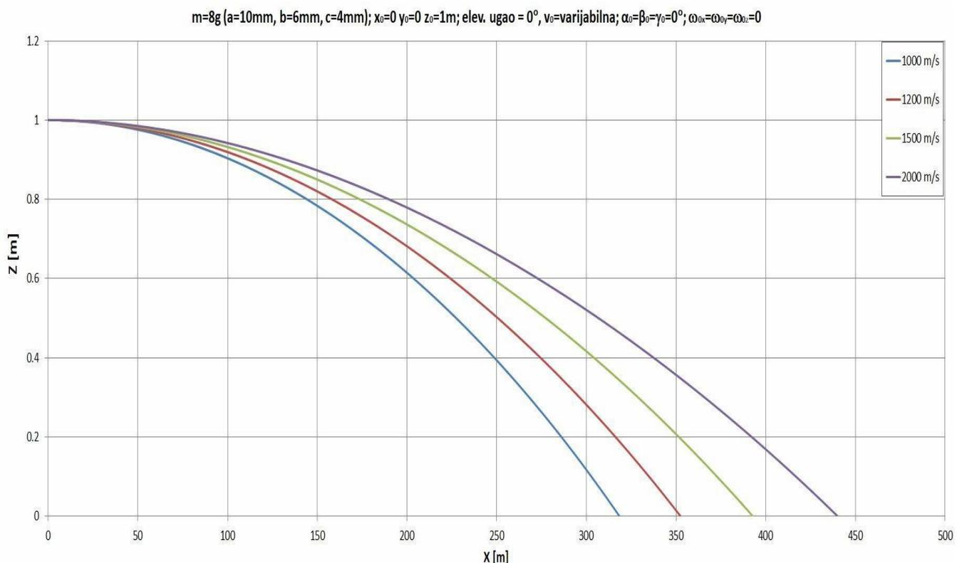
Figure 15. Influence of the initial translational velocity on a fragment trajectory
