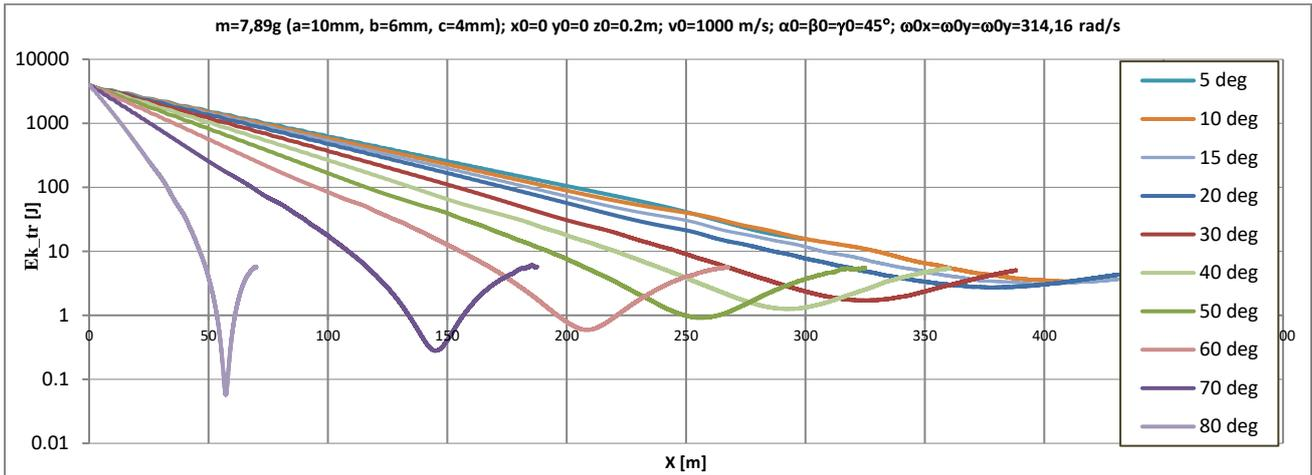
Figure 13. Decrease of translational kinetic energy for a fragment with a mass of 7.89 g for different elevation angles - logarithmic scale
