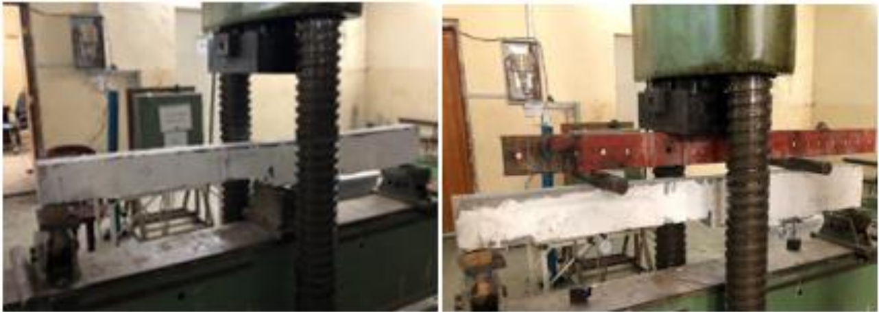
Figure 3. Beam test setup
