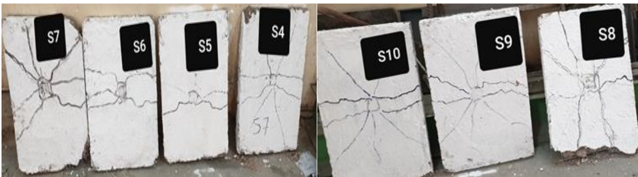
Figure 7. Failure pattern and failure zone shape
