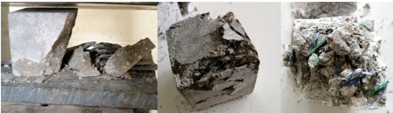
Figure 7. Mode of failure under compression force
