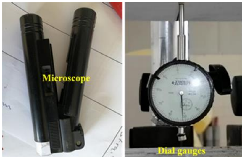
Figure 3. Microscope and dial gauge that were used to recorded crack width and deflection, respectively
