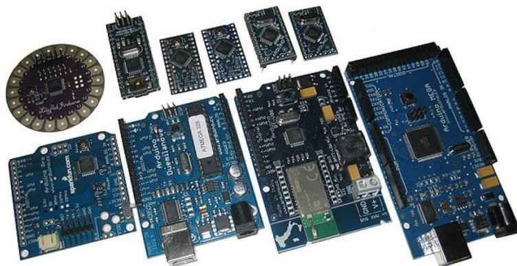
Figure 6. Range of Arduino boards [15].
