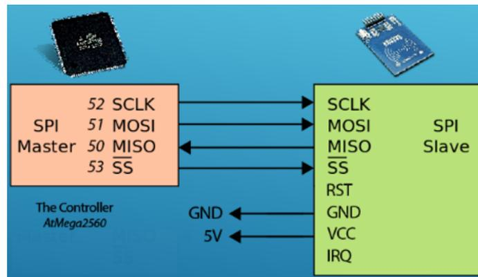
Figure 4. ISPI bus used in our implementation.
