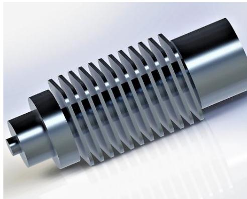
Figure 1. Rendered solid model of the heat sink
