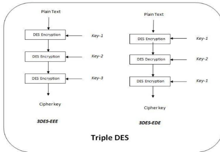
Figure1. flowchart of 3DES algorithm[9]
