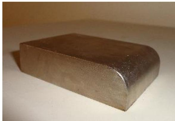
Figure 3. Steel rounded broad crested weir
