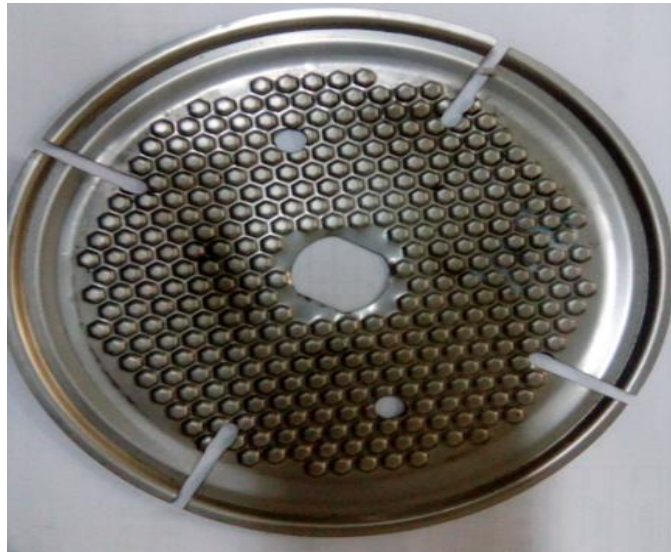
Figure 13. The obtained part after printing in press
