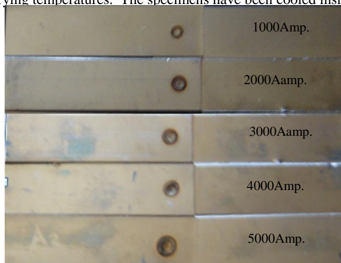
Figure 5. Photograph of spot welding specimens at varying values of welding current
